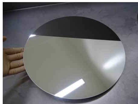
Figure 8. 3mm thick, 300mm diameter sample used for stress measurement
