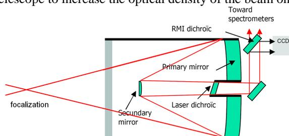
Fig. 3 Optical design of the telescope
