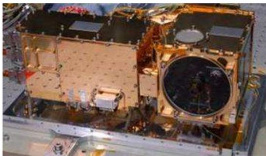
Fig. 2 CHEMCAM Mast Unit Flight Model (Image credit CNES)
