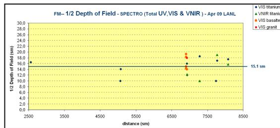
Fig. 9 : ½ LIBS DoF versus distance to target given by spectrum criteria
