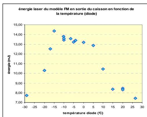
Fig. 4. Energy received by the target versus laser temperature.
