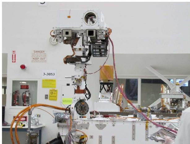
Fig. 1 view of CHEMCAM Mast Unit on the MSL Rover (Image Credit: NASA/JPL-Caltech)
