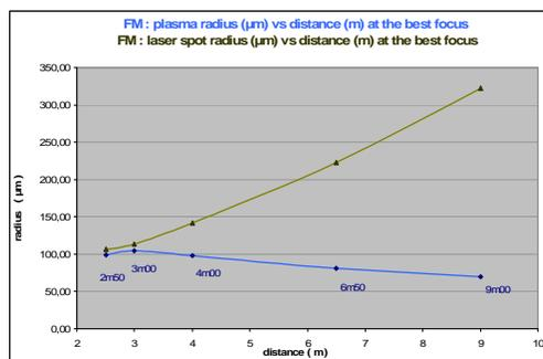
Fig. 6 : Radius of the laser spot and the plasma versus distance at the best focus.
