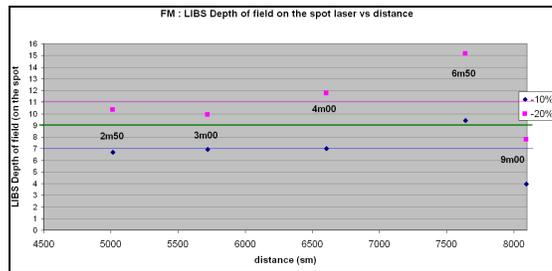
Fig. 8. ½ LIBS DoF versus distance given by Laser ED criteria
