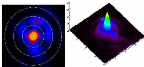
Fig. 5 : Concentration of energy measured on the target at 9 m.
