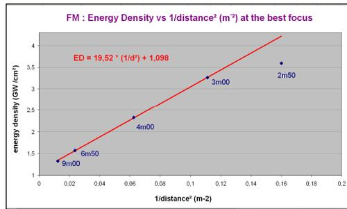
Fig. 7: Energy Density deposited on the target versus 1/distance<sup>2</sup>.
