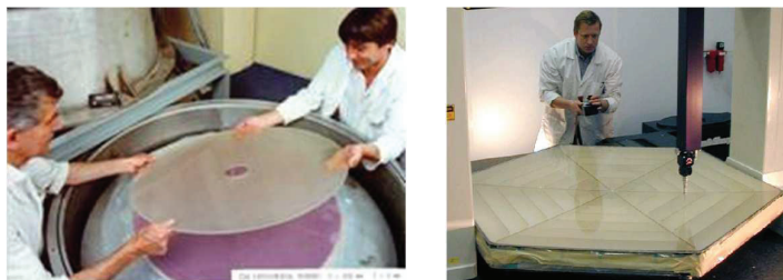
Figure 16. Left: Semi-passive mirror for ESA study and Right: Hybrid mirror with thin shell on CFRP structure
