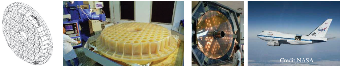
Figure 4. The SOFIA primary mirror design, machined, integrated, in flight
