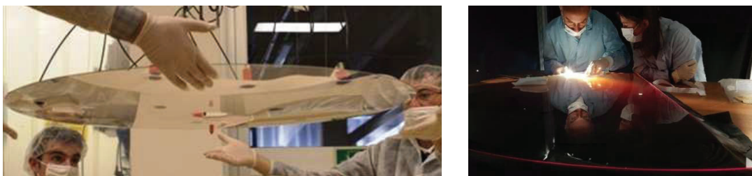
Figure 15. Left: Thin glass shell for VLT M2 AO Unit - Right: The first petal shaped thin shell for ELT M4 Unit
