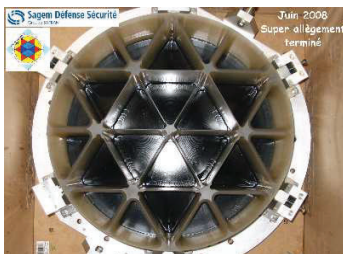
Figure 9. Ultra lightweighting breadboarding activities
