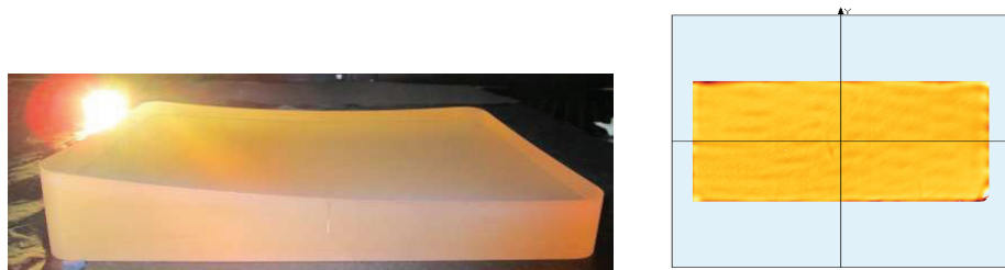
Figure 11. Severe freeform polishing demonstration to high performance (14 nm RMS residual surface error)
