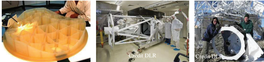
Figure 6. The Sunrise 1 m primary mirror – The telescope prepared at DLR – The mirror recovered after landing
