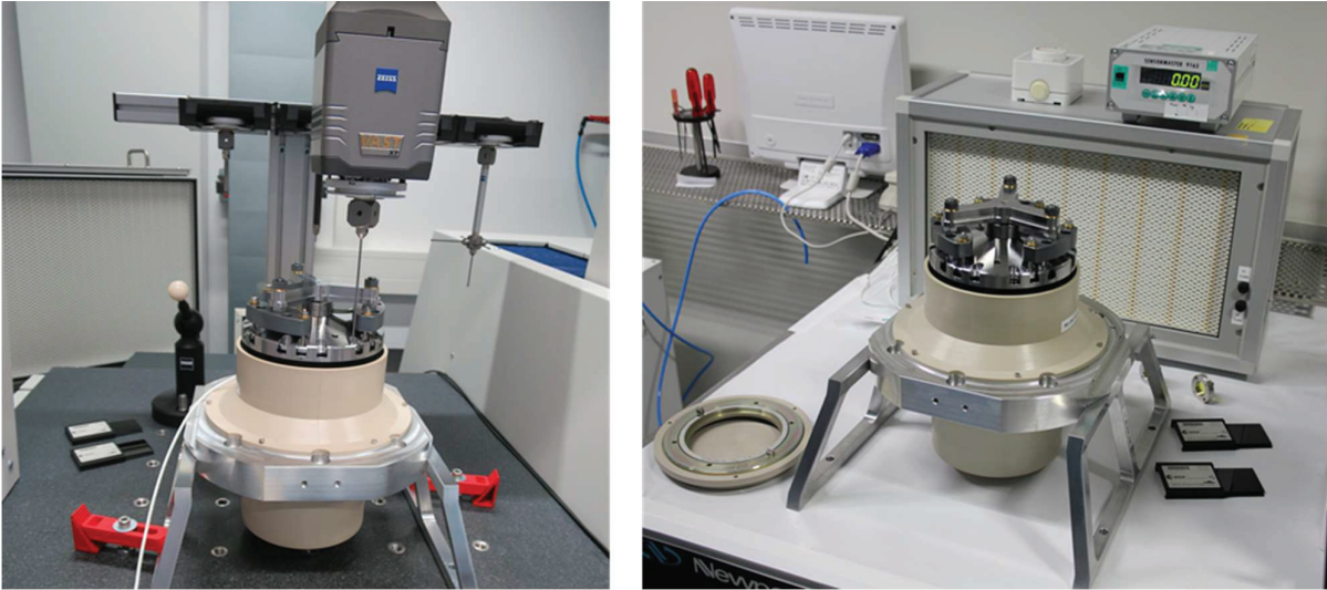
Figure 8. Clamping of the TOA-PFM optical module, Left: probing the lens stack in relation to the tube flange, Right: clamping setup for the final locking of the TOA-PFM
