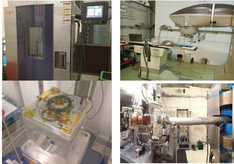
Figure 3-5. Pictures during photonic components level characterization. Temperature cycling (left up), mechanical shock (left down), TID (right up) and Proton test (right down)
