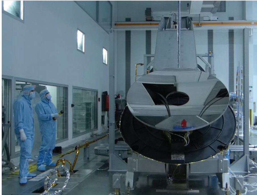
Figure 3-10 – TANGO zerodur M1 mirror in testing sequence at Thales Alenia Space Cannes
