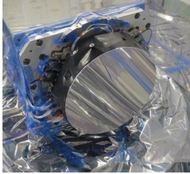
Figure 3-6 – MTG MIFCI coated mirror during tests
