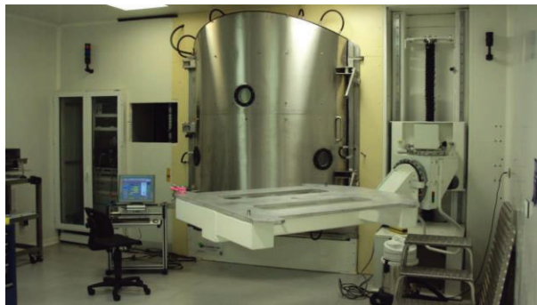
Figure 3-1 – Thales SESO STEP coating machine, 1.7 m capable
