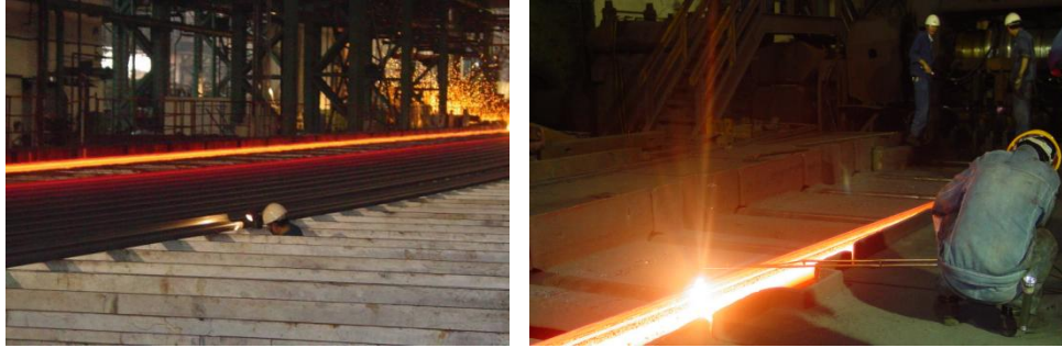
Figure 1. Manual visual method for the detection of defects on the upper and lower surfaces of heavy rails
