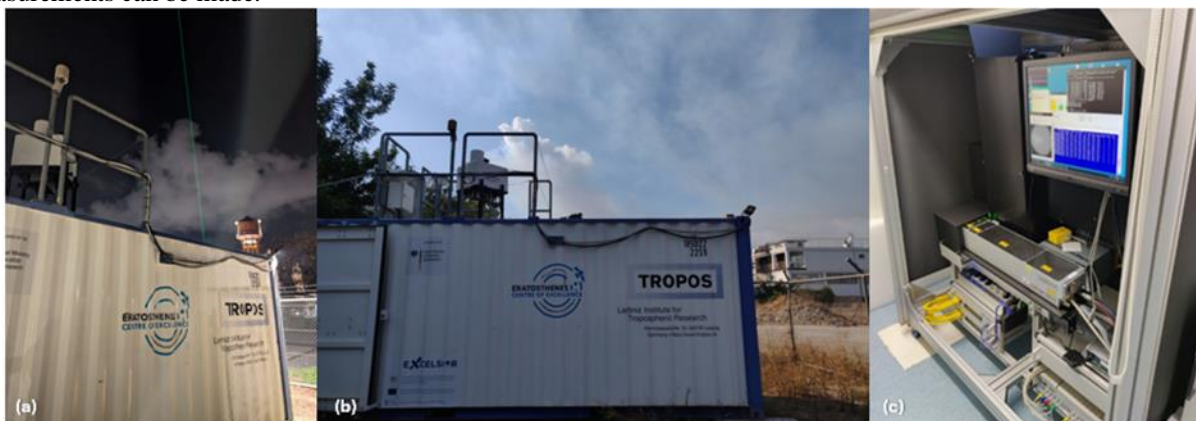
Figure 1. (a, b) CARO station (34.677°N, 33.0375°E), (c) PollyXT lidar main subsystems.
