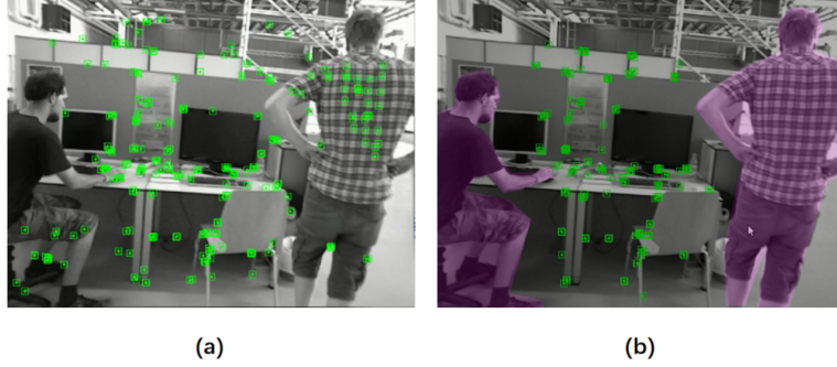
Figure. 4. Dynamic feature point screening strategy. (a) All extracted feature points (b) Static feature points remaining after removal by the dynamic feature point algorithm.
