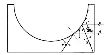
Figure 6. Light polarization by scattering when it is seen perpendicularly to the direction of the incident beam.
