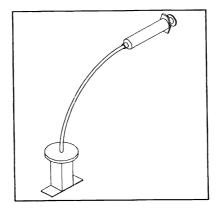
Figure 2. Vacuum system with a cell and a syringe.
