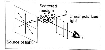
Figure 5. Linear polarization by scattering at 90°.
