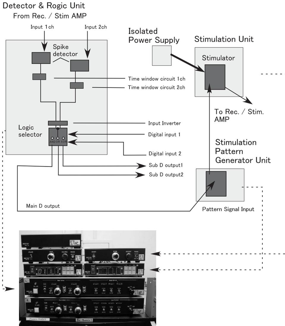
**Figure 1.** Real-time feedback stimulation system. This system composed by 3types of unit and the units can be combined one by one. Each "detector and logic unit" has 2 window discriminators and a logic calculator. The unit outputs trigger signal to "stimulation pattern generator unit". User can determine the frequency and the number of pulses using the pattern generator unit. The stimulation unit is an isolator.
