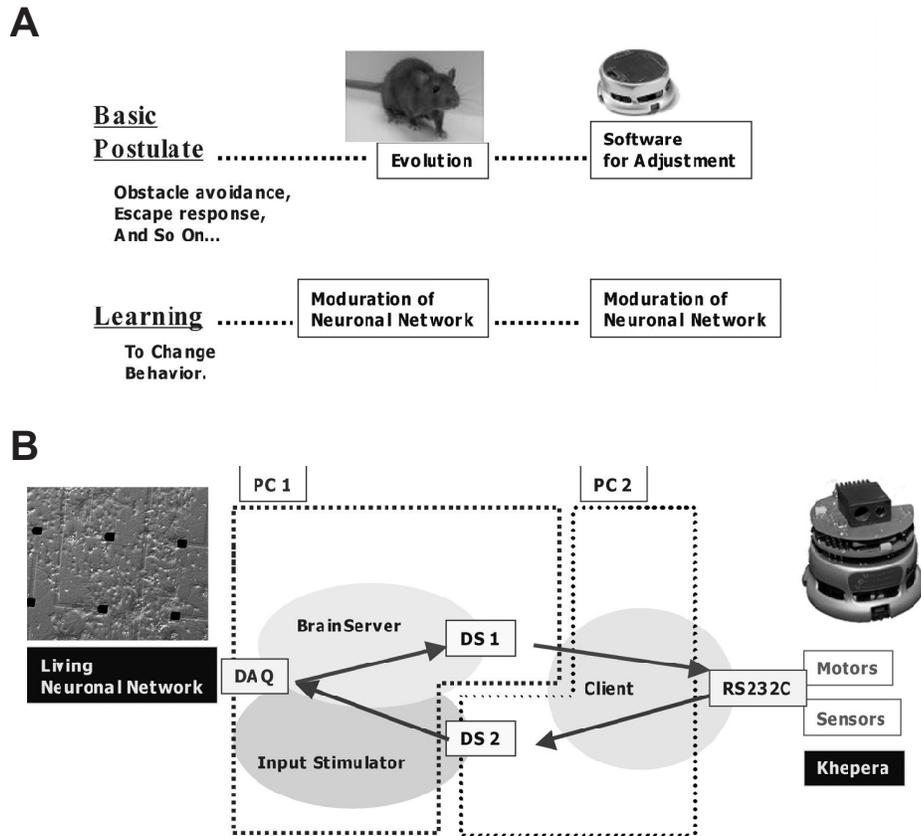
**Figure 9.** Living neuronal network with moving mini robot. **A.** Comparison between a creature and a robot with living neurons. **B.** Scheme of "Living Brain Robot System" .
