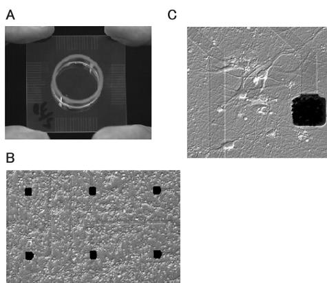
**Figure 2.** A.Culture dish with 64 planer electrodes (MED probe). B.Cultured neuronal network on multielectrode array. The black squares are electrodes. 200  $\mu$  m C.Expanded image of neurons. Black bar indicates 50  $\mu$  m. Neurons re-constructed complex networks *in vitro*.
