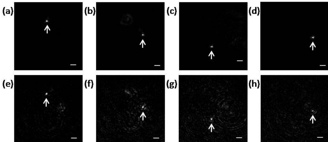
Fig. 7. Images of SHRIMPs embedded in PDMS. (a)-(d): SHG images of SHRIMPs on four different planes, focusing by moving the optics with a conventional microscope. (e)-(h): Holographic reconstructed images of SHRIMPs on four corresponding planes, focusing by digital reconstruction. The relative depths of these four planes are 0, 9.4, 17.2, and  $20.3\ \mu\text{m}$  respectively. Scale bars are  $2\ \mu\text{m}$ .
