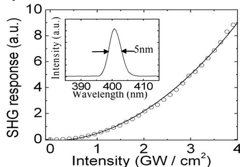
Fig. 2. Quadratic SHG response of  $BaTiO_3$  nanoparticles versus the excitation peak intensity. The circles show the experimental results while the line is the quadratic fit. Inset: optical spectrum of the SHG signal.
