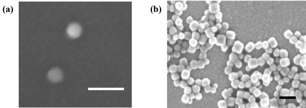
Fig. 1. The SEM images of  $BaTiO_3$  spherical nanoparticles. (a) 30 nm  $BaTiO_3$  nanoparticles. The scale bar is 100 nm. (b) 90 nm  $BaTiO_3$  nanoparticles. The scale bar is 200 nm.
