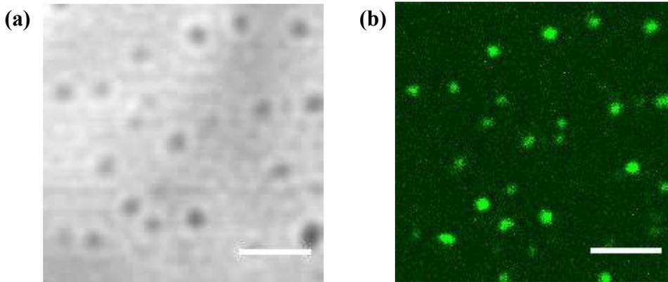
Fig. 3. Confocal images of BaTiO<sub>3</sub> nanoparticles deposited on a glass substrate. (a) Transmission image. (b) SHG image. The scale bars are 5 μm.
