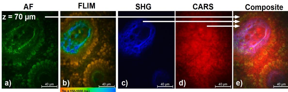
Fig. 4 The multiphoton/CARS tomograph MPTflex-CARS with its 4-detector unit provides within one optical section simultaneously autofluorescence (AF), FLIM, SHG, CARS, and overlay information<sup>18</sup>.
