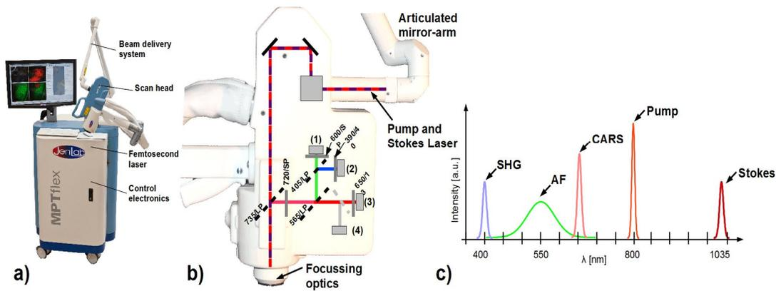
Fig. 2 Multiphoton tomograph (a) with scan head with four-detector arrangement (b) and spectrum of excitation and detection signals (c)<sup>18</sup>.
