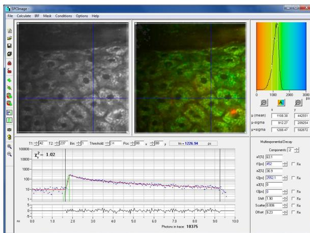
Fig. 5 Optical section of in vivo human skin with fluorescence lifetime information and counts of 9 pixels = binning 1 (n=10,375).
