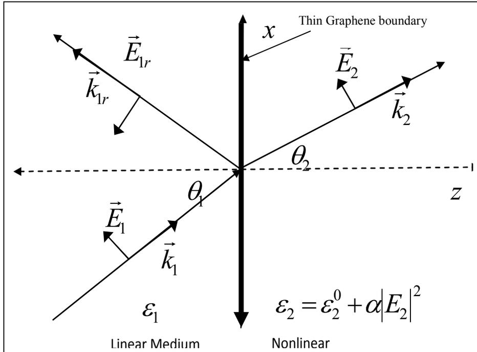
Figure 1. Transverse Magnetic (TM) incident, reflected, and transmitted Electric Fields.
