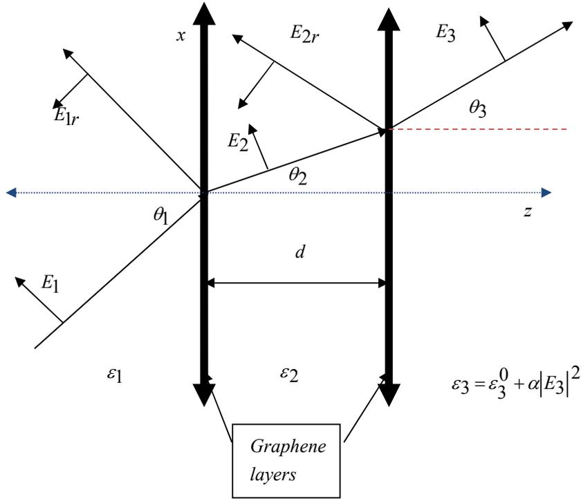
Figure 4. The multilayered waveguide with two thin graphene layers.
