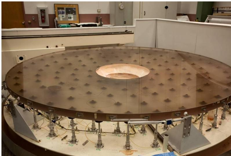
Figure 24. The 4.3-meter-diameter primary mirror for the Discovery Channel Telescope.
