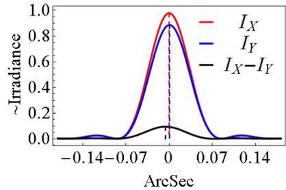
Figure 11. The cross-section profiles of the  $I_X$  and  $I_Y$  PSF images, one for each polarization and the profile of their difference are shown in red and blue in arc seconds from the center of the PSF. The black line shows Stokes  $Q$  image, the difference between the two PSFs.
