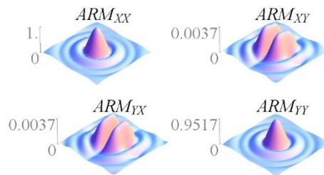
Figure 7. The absolute value of the amplitude of the 2×2 **ARM** at an on-axis field point is shown for the example telescope of Figure 2 normalized by the peak of the *XX*-component.
