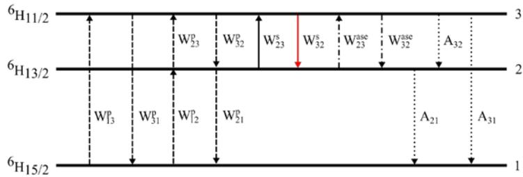
Figure 2. Diagram of Dy<sup>3+</sup> energy levels and transitions [from Ref.45]. The 4.5 micron transition, in red, is between H<sub>11/2</sub> and H<sub>13/2</sub> levels
