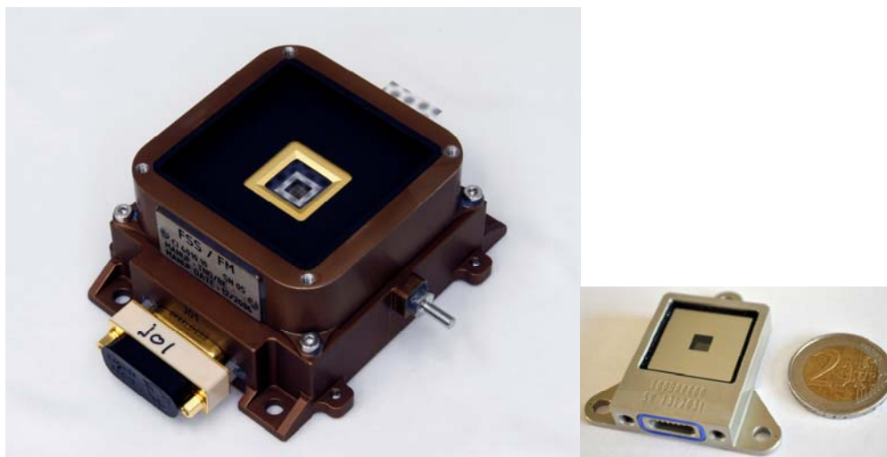
Figure 5 Moog Bradford (TNO) FSS and BiSon 64 sensors
