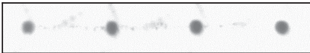
Fig. 8. Output of the 1 \times 4 power splitter imaged with an IR-camera.
