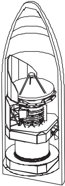
Figure 1: FIRST and PLANCK merged under Ariane 5 fairing.
