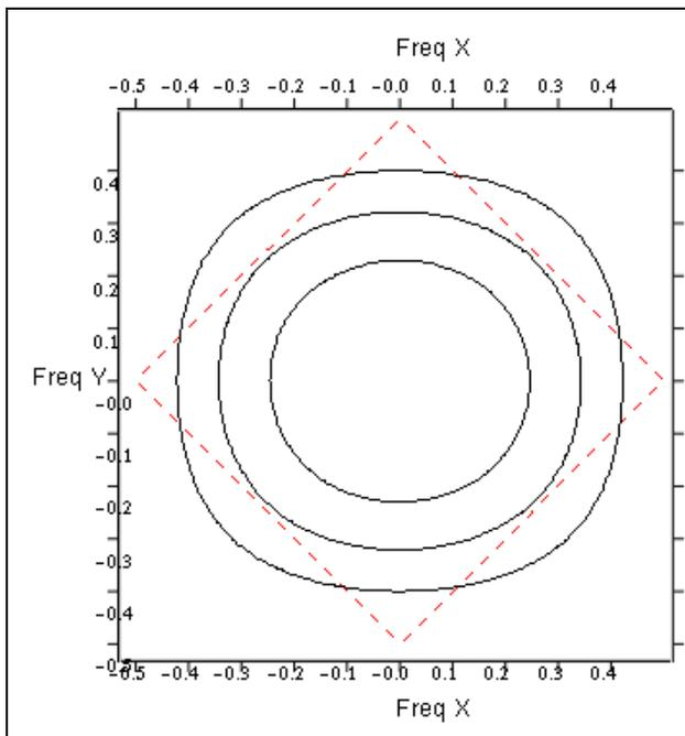
Fig 1.b MTF and reciprocal cell for SPOT 5 THR mode
