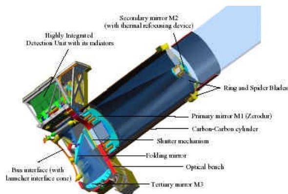
Figure 6. PLEIADES -HR instrument exploded view.
