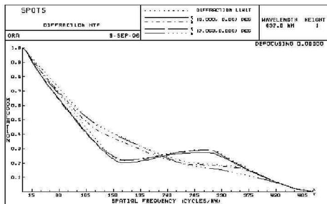
Figure 3. Theoretical diffraction MTF of the HRG telescope
