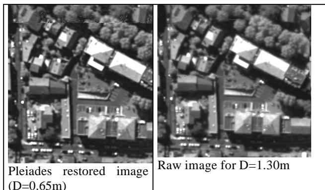
Figure 5 : enhancement due to the restoration
