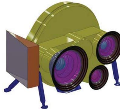
Fig. 4 : The Opto-mechanical Assembly gathering the objectives, the filter wheel and the detection units. On the left there is the SWIR radiator and its earth shield
