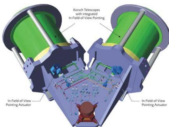
Figure 1. Single test mass payload configuration for LISA. The inertial sensor is located on a single optical bench and similar to the LISA Pathfinder
