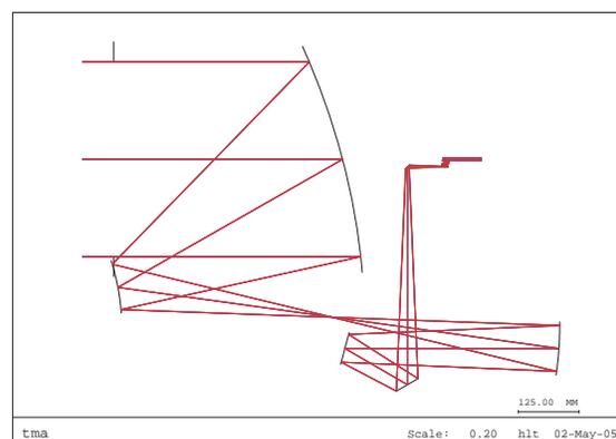
Figure 4. Optical layout of the asymmetric Korsch in Figure 3. The in-field beam steering is walking the beam perpendicular to the plane.
