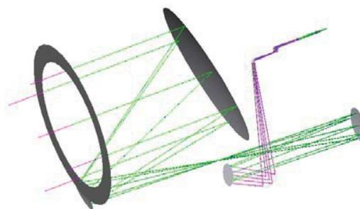
Figure 3. Asymmetric Korsch all reflective three mirror design at  $WFE < \lambda/20$  and suitable pupil plane locations capable for in-field guiding by  $\pm 1^\circ$
