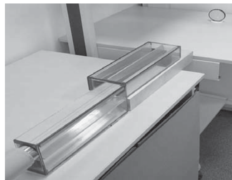
Fig. 14: Test parabolic KB X-ray imaging system based on parabolically shaped glass foils with dimensions of 300 x 100 x 0.3 mm. The complete KB
