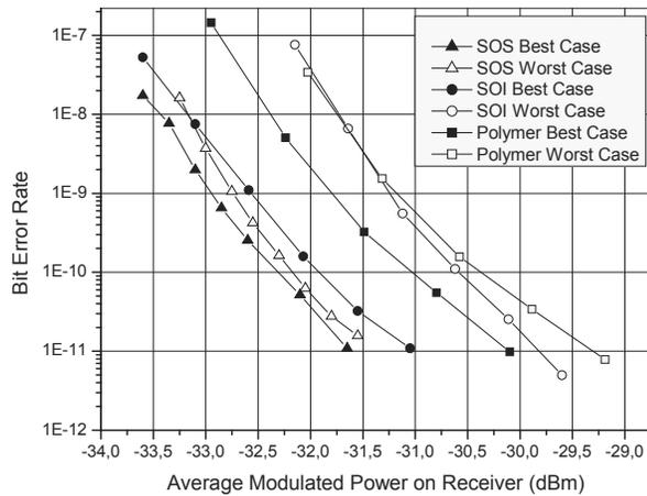
Fig. 3. Back-to-back BER measurements for the SOS, SOI and Polymer AWGs.
