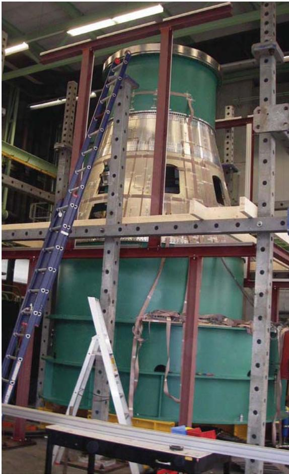
Fig. 10. Vega Interstage 1/2 installed on test bench at TNO, Delft.
