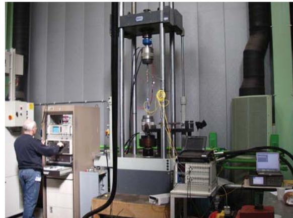
Fig. 6. Setup for stresses up to 100 kN at TNO, Delft.
