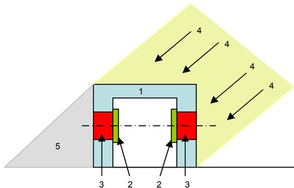
**Figure 3 Schematic presentation of sun blocking. The numbers in the figure 3 represent: 1 Housing, 2 Detector, 3 Aperture, 4 Sunlight and 5 Shade.**
