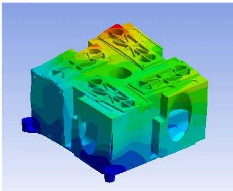
**Figure 5 First mode of Natural frequency. This picture shows a torsion movement around one of the mounting points.**
