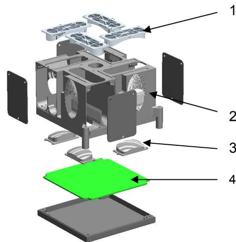
**Figure 4 Exploded view of MABS. The number in figure 4 represent: 1 Upper mirror, 2 Monolithic housing, 3 lower mirror, 4 Electronics**
