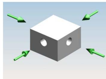
Figure 2 Multi-aperture layout. Four apertures are placed in a orthogonal pattern.
