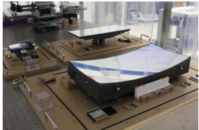
Fig. 13. Sentinel-2 mirrors after coating in cleanroom
