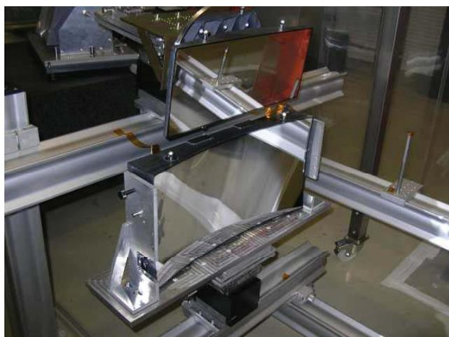
Fig. 15. M1 and M3 mirrors on the bench
