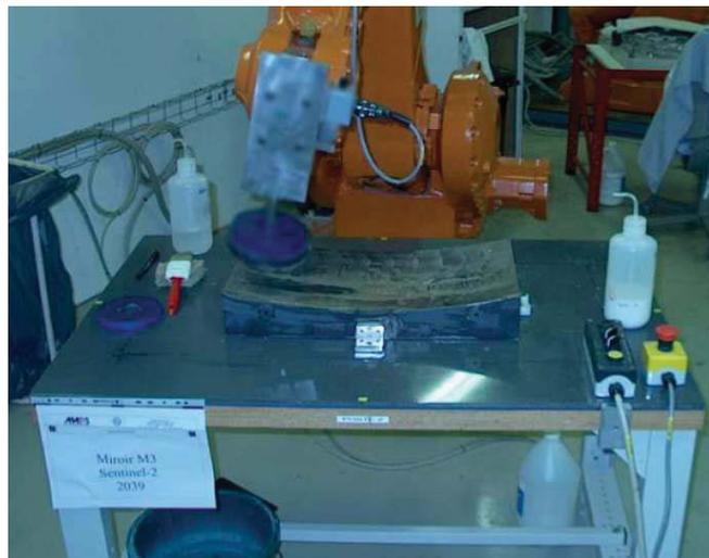
Fig. 3. Robot lapping of M3 mirror
