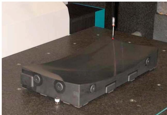
Fig. 4. CMM measurement on M3 mirror
