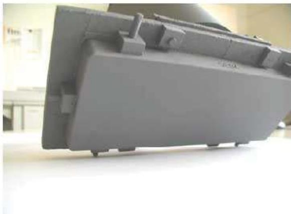
Fig. 2. Mirror blank after CVD cladding
