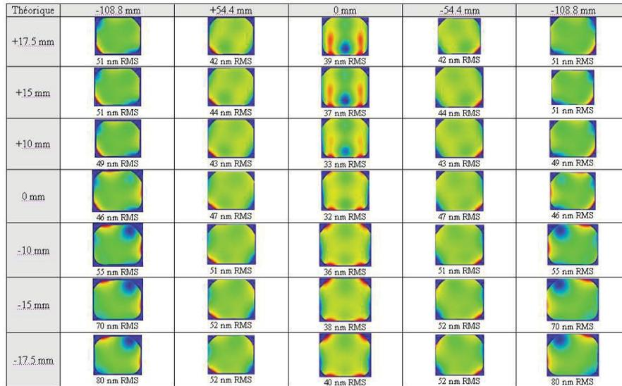
Fig. 17. Telescope image quality (design values)
