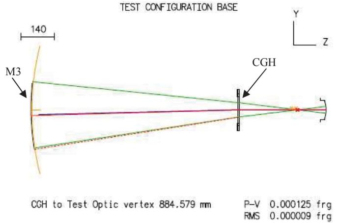
Fig. 8. M3 test configuration
