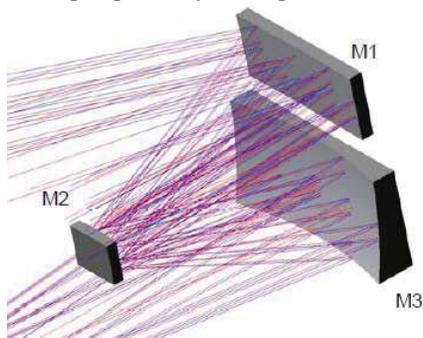
Fig. 1. Telescope optical lay-out
