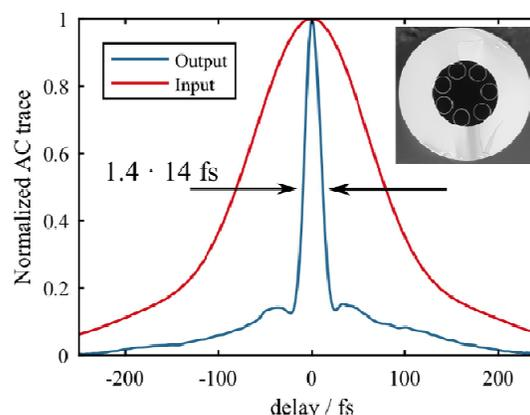
Fig. 1. Measured AC traces before (red) and after the nonlinear compression (blue) Inset: Cross-section of the antiresonant hollow-core fiber.
