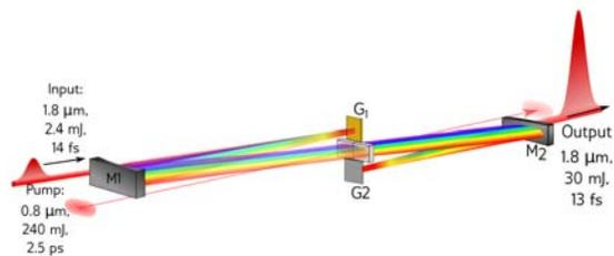
Fig. 1: Layout for high energy Frequency domain Optical Parametric Amplification.
