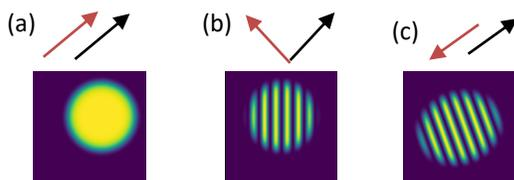
Fig. 2. Simulated interference patterns of (a) common MZI, (b) inverted MZI (Ref. 2), and (c) Rotated MZI.
