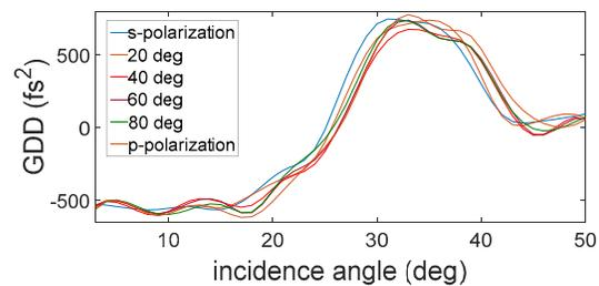
Fig. 1 Measured Group Delay Dispersion at 800 nm
