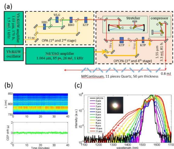
Fig. 1 (a) OPCPA setup. (b) CEP measurement of the front-end 1.55  $\mu\text{m}$  pulses in a f-to-2f interferometry. CEP shifts with a fluctuation of 257 mrad acquired for 40 minutes. (c) Spectra of the pulses from OPCPA directly, passing through air only, and through different numbers of quartz plates. All the spectra are set to normalize its maximum value. Inset figure: Photographic image of MPC taken by a visible camera right after the 11<sup>th</sup> quartz plate.
