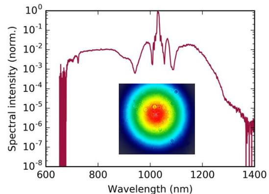
Fig. 1. Measured spectrum of the HR1 laser output. The inset shows the collimated beam profile after the second compression stage.
