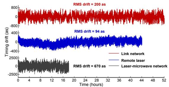
Fig. 2. Long-term timing drift results for the laser-microwave network<sup>4</sup>.
