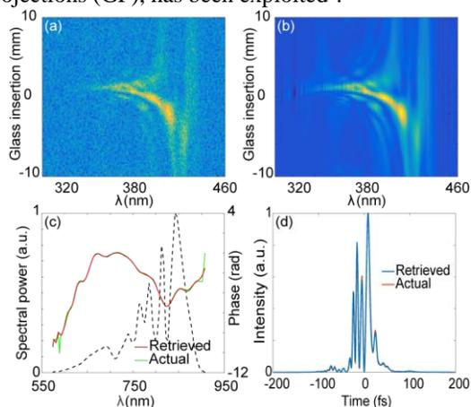
Fig. 1. (a) The d-scan trace with 10% noise, (b) the retrieved trace, (c) pulse in wavelength domain, and (d) in time domain, showing excellent agreement.
