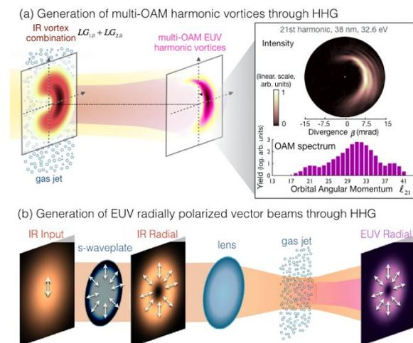
Fig. 1. (a) Generation of multi-OAM beams through HHG, using two IR drivers with different OAM<sup>4</sup>. (b) Generation of EUV radial vector beams through HHG. The harmonic emission is composed of a train of radially polarized attosecond pulses<sup>6</sup>.
