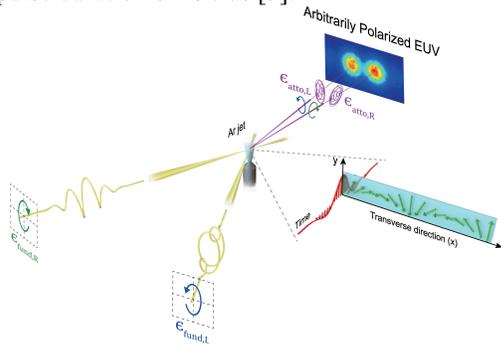
**Fig. 1 (a)** Schematic of the experimental setup. The inset shows the electric field distribution on the focal plane – local E-field vectors rotating crossing the transverse direction  $\hat{x}$ .
