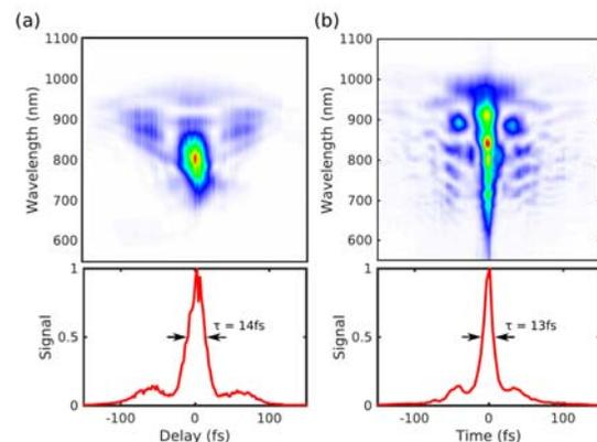
Fig. 2 : SHG-FROG Traces obtained (a) before and (b) after amplification, with their respective autocorrelation traces. Reconstruction demonstrates sub-12 fs pulses.
