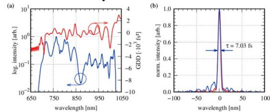
Fig. 2. OPCPA pulse characteristics, measured with SPIDER. (a) Fundamental spectrum and reconstructed GDD, (b) reconstructed temporal pulse shape (blue) and Fourier-transform-limited pulse of 6.6 fs (red).
