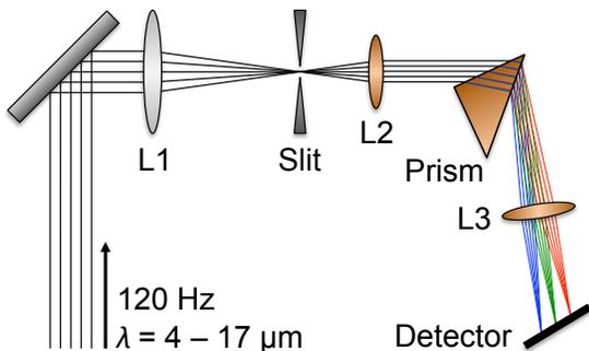
Fig 1. Optical design of the prism spectrometer. Mid-IR laser pulses are generated using a commercial OPA laser source (HE-TOPAS, Light Conversion).
