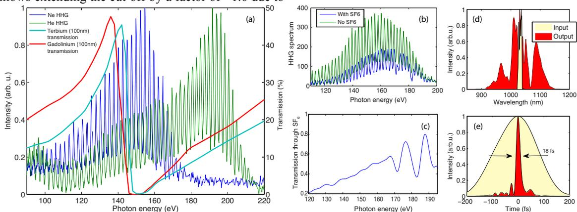
**Fig. 1** (a) Spectra of high-order harmonics generated in helium and neon driven by the compressed 20 fs 1030 nm pulses; For reference, X-ray transmission data of Tb and Gd magnetic materials from a database is shown; (b) shows the measured HHG spectrum transmitted through SF<sub>6</sub>; (c) transmission spectrum through SF<sub>6</sub> obtained from the spectra shown in (b); (d) and (e) spectra and temporal profiles from FROG characterization of the post-compressed 18 fs pulses.
