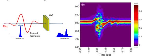
Fig. 2. THz induced XPM giving rise to extreme spectral broadening of the nIR probe pulse.
