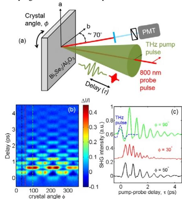
Fig. 1. (a) Experimental setup for THz-pump, SHG-probe measurements. (b) The THz-induced change in the SHG versus delay  $\tau$  and crystal angle  $\phi$ . (c) The THz-induced SHG change at a few different angles. Data taken from [3].
