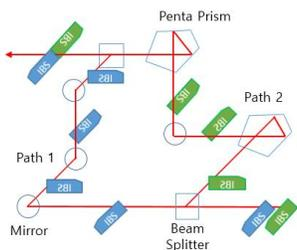
Fig. 1. Schematic layout of the Rotated MZI. The beams through path 1 and 2 are rotated 180 degrees from each other.
