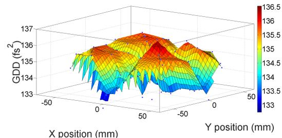
Fig. 2 Measured Group Delay Dispersion over 16 cm aperture mirror
