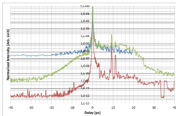
Figure 1: Contrast measurements: Blue line Ti:Sa stage alone; Green line Ti:Sa stage and OPCPA stagewithout XPW, Red curve Ti:Sa stage with XPW and OPCPA stages.
