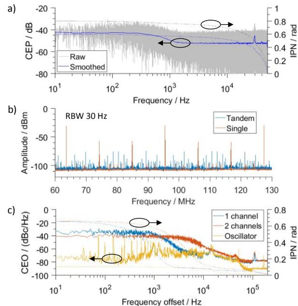
Fig. 1. (a) Single-shot stereo-ATI measurement in a single-channel regime. (b) Tandem AOMs as pulse pickers, picking factor 2. (c) CEO noise of the CPA
