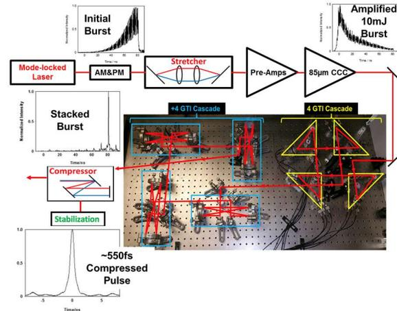
Fig. 1: Coherent pulse stacking amplification system schematic. The initially modulated burst before amplification as well as the amplified 10mJ burst are shown. The layout for the GTI pulse stackers is given with the beam path through the GTIs. Also included is the autocorrelation trace of a compressed amplified burst giving 550fs pulses. Additionally an image of a stacked burst of 81 pulses is shown at the output of the GTI stackers.
