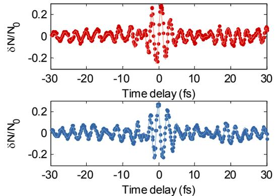
**Fig. 1.** Few cycle laser pulses measured by the TIPTOE method are shown. The modulation of the ionization yield  $\delta N/N_0$  is measured at different CEPs, including the carrier envelope phase (CEP) of the pulse.
