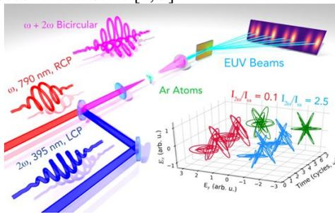
Fig. 1. Experimental scheme for controlling the ellipticity of APTs produced via bicircular-driven CPHHG. Theoretical APTs obtained from CPHHG spectra driven at different intensity ratios of the bicircular field (inset).
