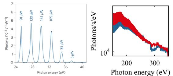
Fig. 2. a) 100  $\mu$ W HHG spectrum. B) Water window HHG with 2  $\mu$ m lasers with (blue) and without (red) a Mylar filter.
