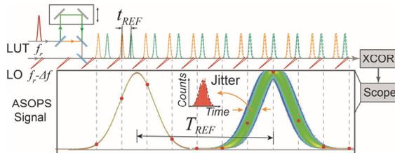
Fig. 1. Concept of timing jitter measurement based on ASOPS.
