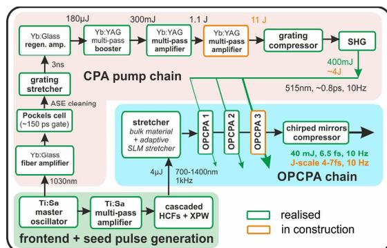
Fig. 1. Schematic layout of the PFS system.
