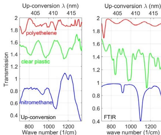
Fig. 1. Static mid-IR transmission measured with 4WM up-conversion (left) and an FTIR (right).
