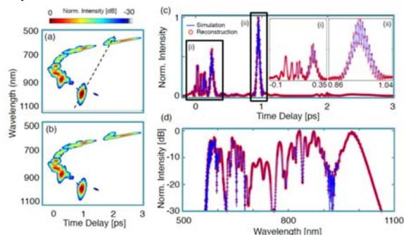
Fig. 2. (a) Simulated; (b) reconstructed spectrogram. (c) Temporal intensity and (d) logarithmic spectrum.
