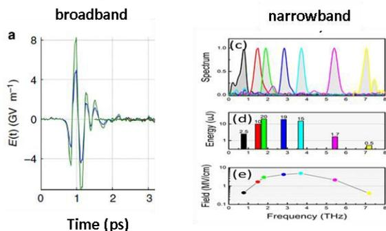
Fig. 1. Broadband, 80 MV/cm single-cycle pulses (left) and narrowband THz radiation (right). The latter is tunable across 0.5-8 THz and offers up to 20 uJ.
