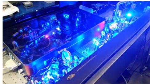
Figure 1. First of its kind, Ti:sapphire oscillator /amplifier pumped with 465nm laser diodes . 3.1 W in the oscillator, and 12W in the cryogenically cooled amplifier producing 3W of amplified power.
