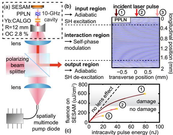
Fig. 1. (a) Straight cavity setup. (b) Fanout + apodized PPLN device. (c) Fluence on the SESAM as a function of pulse energy for different transverse positions of the PPLN with respect to the incident pulse.
