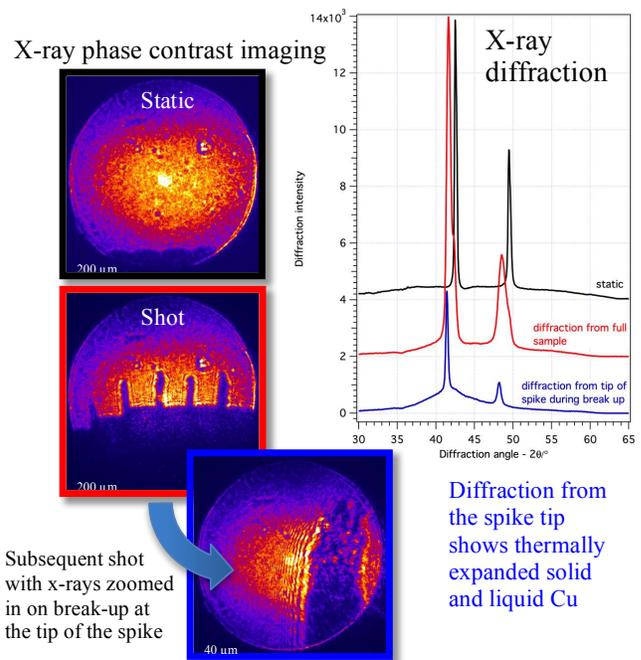
Fig. 1. Concurrent PCI and XRD of materials jets off of a free surface in shock loaded copper conducted at the LCLS-MEC.
