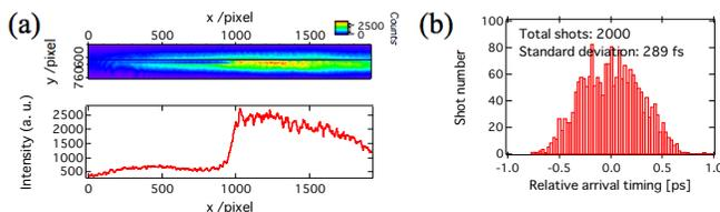
Fig. 2, (a): CCD detector image (top) and horizontal line profile (bottom) of the arrival timing monitor, (b): Histogram of edge variation
