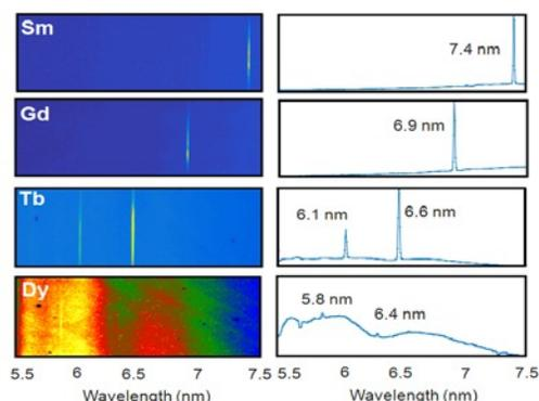
Fig. 1. End-on spectra showing lasing at progressively shorter wavelengths in the  $4d\ S_0-4p\ P_1$  line of nickel-like lanthanide ions, down to  $\lambda=5.8$  nm in nickel-like Dysprosium.
