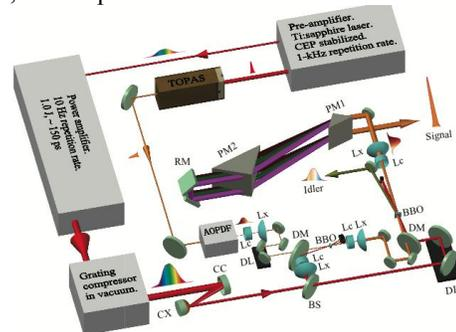
Fig. 2: Schematic of the DC-OPA setup
