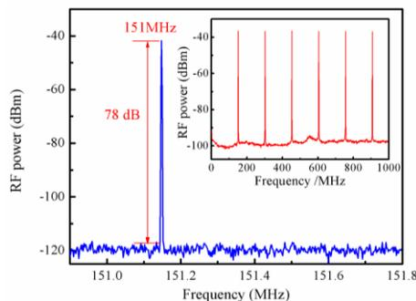
Fig. 1. RF spectrum of fundamental beat note with the RBW of 1 kHz; inset: wide RF spectrum of 1GHz with the RBW of 100 kHz.
