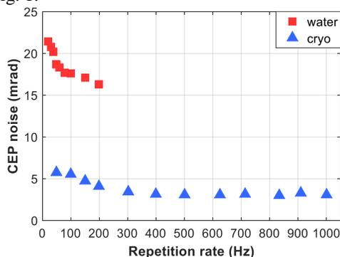
Fig. 1. Thermal originated CEP noise at different repetition rates in a single pass for the water-cooled (red) and cryogenically cooled amplifier (blue).
