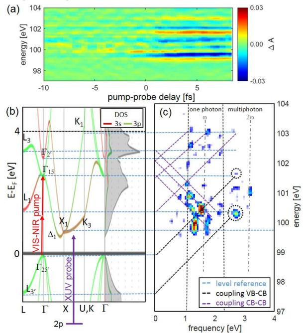
Fig. 1. (a) Transient absorption changes at the silicon L<sub>2,3</sub>-edge. (b) Si band structure and density of states (DOS) indicating critical points and the pump-probe scheme. (c) Fourier analysis of (a) revealing various VB-CB and CB-CB electronic coherences. Only one possible excitation pathway is indicated (b) for clarity.
