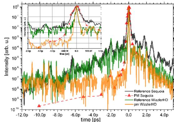
Fig. 2. Measurement of contrast with Sequoia and Wizzler HD with vs. without plasma mirror filtering.
