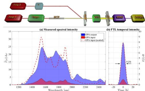
Fig. 2. Few-cycle SWIR OPA scheme (top) and measured amplified spectrum (bottom).
