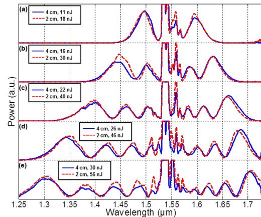
Fig. 2. Output spectra from highly nonlinear fiber at different fiber length (4 cm versus 2 cm) and coupled pulse energy.
