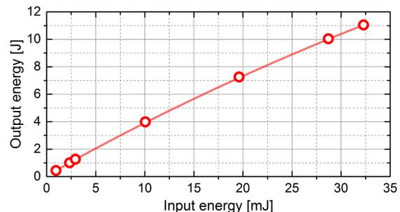
Fig. 1. Energetic performance using  $2 \times 12$  passes at MPA III surpassing 10 J of output energy.
