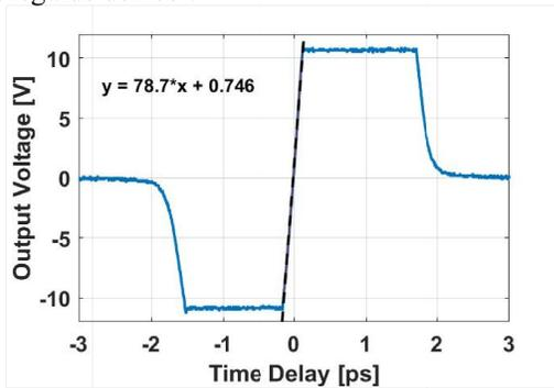
Fig. 2. Measured balanced cross-correlation of the integrated BOC device. The slope of the line is the sensitivity (79 mV/fs).
