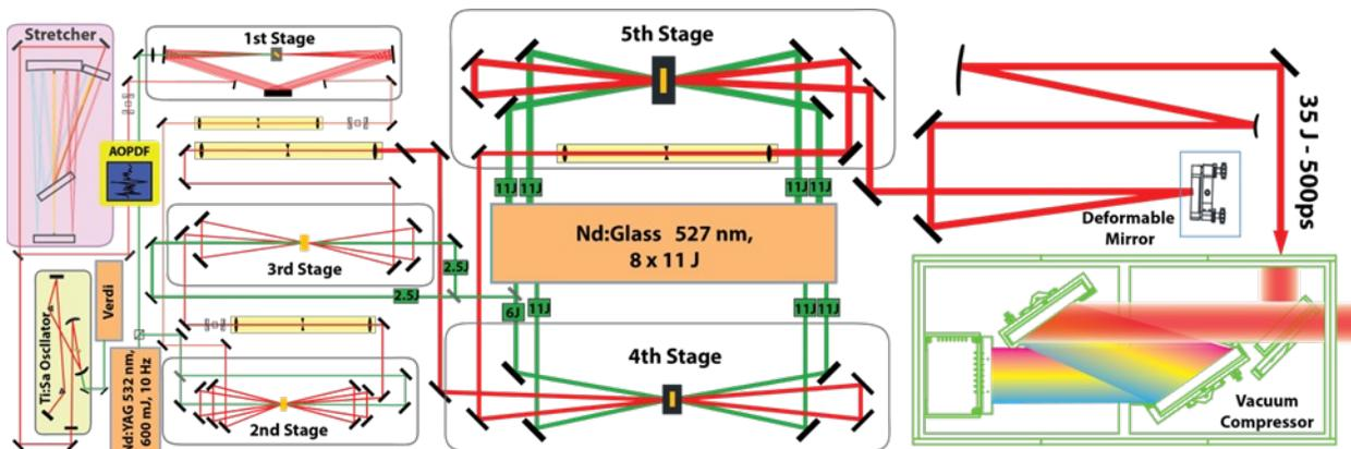
Fig.1. Schematic diagram of the Petawatt-class high repetition rate CPA Ti:Sa laser.
