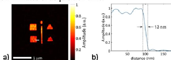
Fig 2. Left: Reconstructed nanoscale image of a test sample. Right: Cut along the small white bar.
