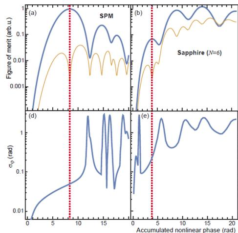
Fig. 1: Numerically simulated figure-of-merit and amplitude and phase variation of the heterodyne signal in the  $f$ - $2f$  interferometer. Left column: symmetric spectral broadening due to self-phase modulation. Right column: asymmetric broadening due to filamentation.
