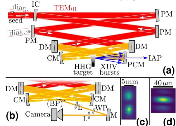
Fig. 1. *a)* Suggested setup for TMG as in [3]. IC: input coupler, diag.: diagnostics, PM: plane highly reflective (HR) mirror, DM: HR delay mirror, CM: curved HR mirror, PCM: pierced curved HR mirror, IAP: isolated attosecond pulse *b)* proof-of-principle experiment. BP: Brewster plate, L: lens, WP: wire-grid polarizer, M: mirror *c)* intensity of the measured mode on the plane mirror and in the focus.
