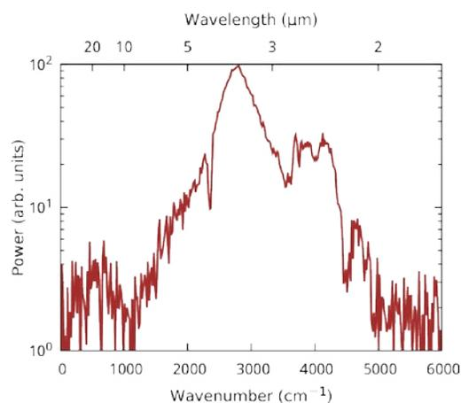
Fig.1. The spectrum of the output from the tapered GeAsSe fiber pumped at 3 mW (300 nJ).
