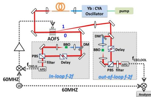
Fig. 1. The experiment setup of Yb:CYA frequency comb with feed-forward scheme. DM: dichroic mirror.
