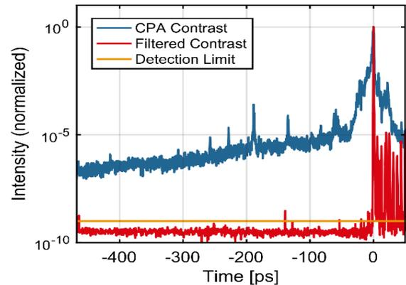
Fig. 2. Pulse contrast of the CPA system before and after SPM contrast enhancement.
