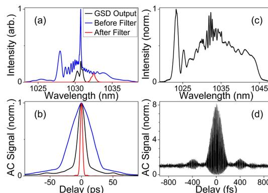
Fig. 1. Spectra and autocorrelations at various points in the Mamyshev regenerator (a-b), and at the compressed output of the system (c-d).
