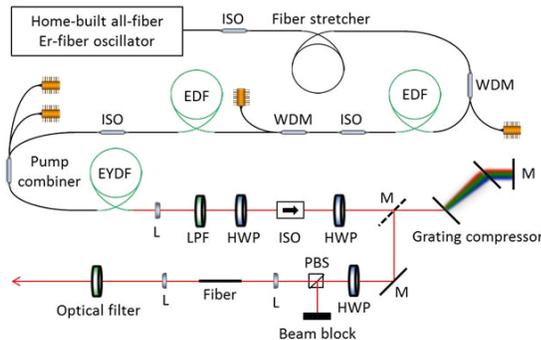
Fig. 1. Schematic setup. WDM: wavelength-division multiplexing, EDF: erbium-doped fiber, EYDF: erbium ytterbium co-doped fiber, L: lens, M: mirror, ISO: isolator, HWP: half-wave plate, PBS: polarization beam splitter, LPF: long pass filter.
