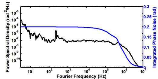
Fig. 3. Integrated phase noise of out-of-loop CEO frequency from 3Hz to 10 MHz.
