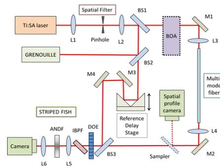
Fig. 1. Delay-scanned STRIPED FISH apparatus and experiment demonstrating its use for measuring MMF pulses.
