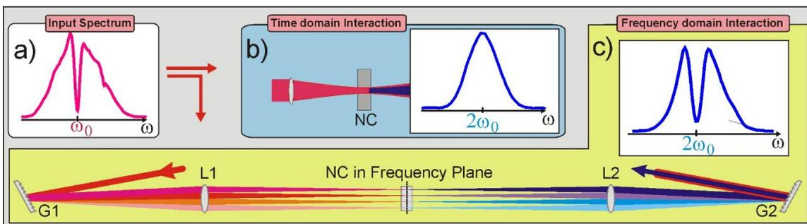
Fig. 1: A shaped input spectrum (a) is frequency doubled either in (b) conventional time domain nonlinear optics (TNO) or (c) via Frequency domain nonlinear optics (FNO). The convolution of different frequencies in TNO (b) leads to a smoothing of the input function while in FNO the shape is preserved since the mutual frequency crosstalk is turned off. This decoupling permits a transfer of arbitrary phase functions. NC: nonlinear crystal.
