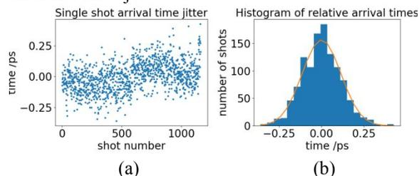
Fig. 2. (a) Relative arrival times of 1142 consecutive single X-ray pulses measured in a  $15 \mu\text{m}$  liquid flat sheet water jet. The distribution (b) of these arrival times has width of 230 fs FWHM.
