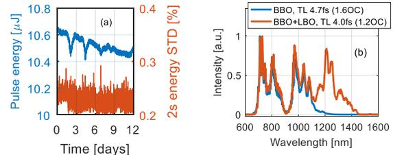
Fig. 2. (a) DFG pulse energy and energy stability (b) Spectra of pulses produced by BBO and BBO+LBO-based OPCPA frontends.
