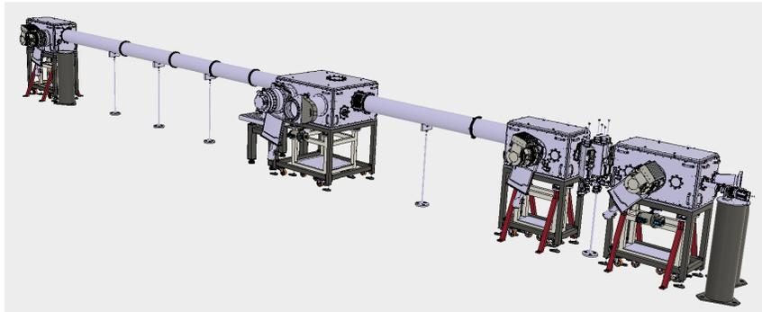
The HHG Beamline has been designed also to accommodate two parallel driving lasers, generating two parallel XUV beams. To our knowledge, this is the only HHG beamline that can generate such a broad spectrum at such high intensities.
