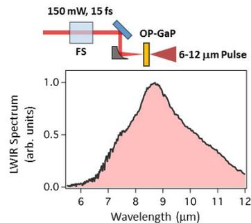
Fig. 2. Experimental layout and resulting LWIR spectrum generated from the 15 fs signal pulse.
