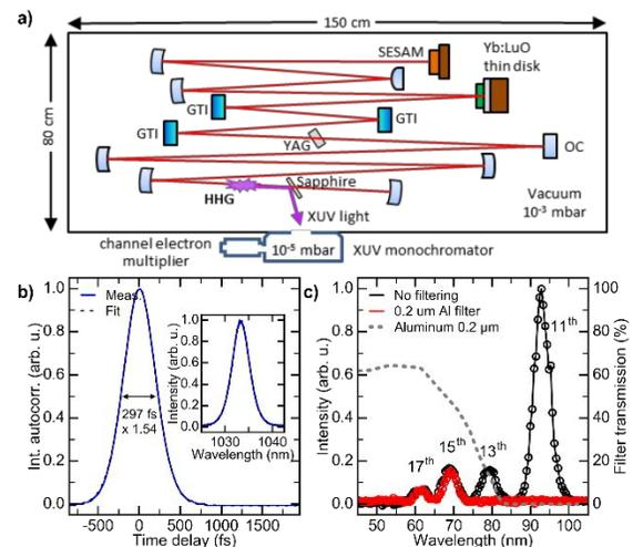
Fig. 1. Experimental setup (a), laser pulses intensity autocorrelation trace and optical spectrum (b), XUV light spectra (c).
