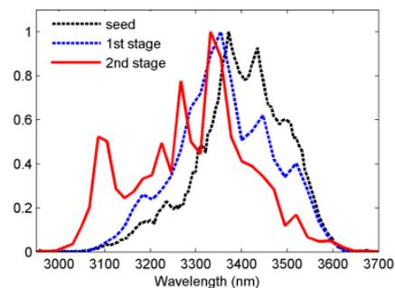
Fig. 2. Spectra of seed (black-dashed) and after the first (blue-dashed) and second (red-solid) stages of the DC-OPA system.
