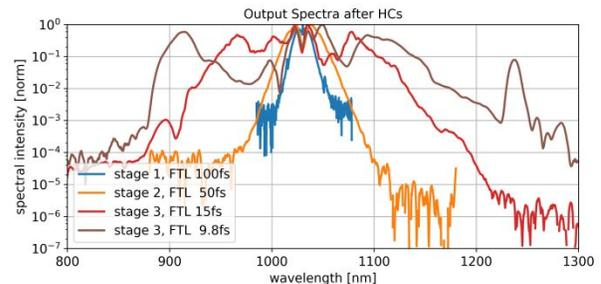
Fig. 2 Spectra after broadening stages
