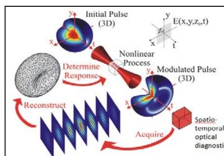
Fig. 1. Conceptual utilization of pulse characterization as an experimental tool. Estimation of the pulsed field before and after the interaction enable full characterization of the system itself.
