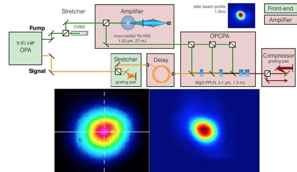
**Fig. 1.** Top) Schematic representation of the OPCPA system. Bottom left) 1.03 $\mu$ m pump profile, bottom right) 3.1 $\mu$ m idler profile.
