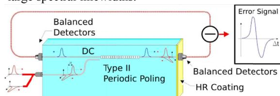
Fig. 1. A schematic of the waveguide-based BOC
