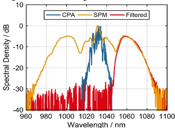
Fig. 1. Spectrum of CPA-signal, which is broadened by SPM and filtered.
