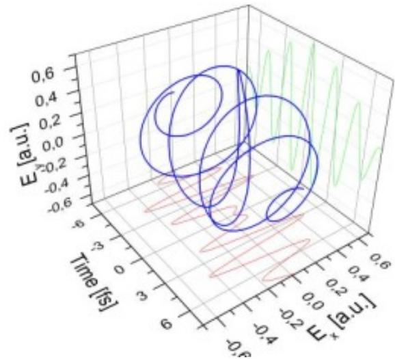
Fig. 1. The field of a polarization-gated few-cycle pulse (blue) reconstructed from two orthogonal projections (red, green) measured experimentally.
