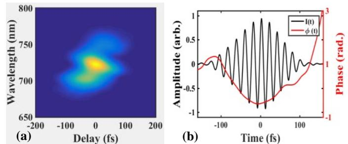
**Figure 1** Example XFROG results for a few-cycle LWIR field
