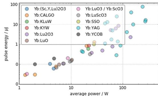
Fig. 2. Overview of modelocked thin-disk laser technology: pulse energy versus average power of laser systems demonstrated up to date.
