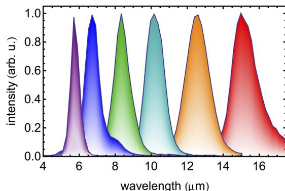
Fig. 2. Pulse spectra obtained from our mid-IR OPA source measured using the prism spectrometer
