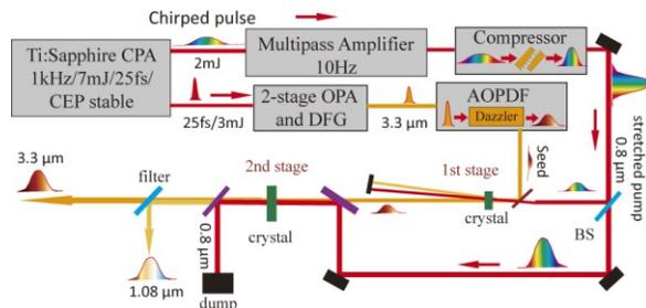
Fig. 1. Experimental setup of MIR DC-OPA.
