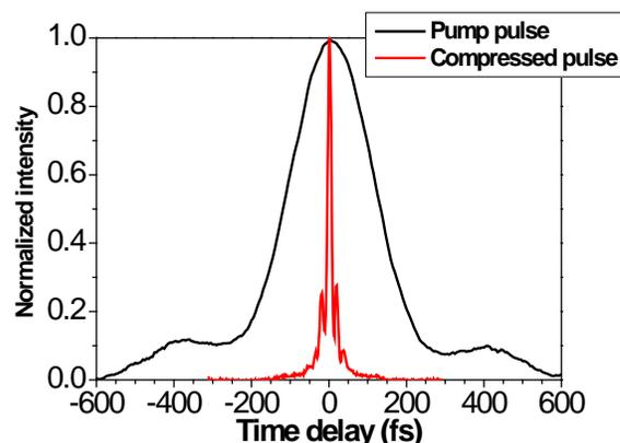
Fig. 1. Normalized autocorrelation of the input pump pulse (185 fs) and the compressed pulse (9 fs) after the Ar-filled HCF (1.73 bar Ar) and chirped mirrors.
