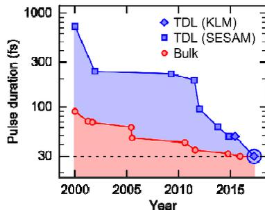
Fig. 1. Evolution of minimum pulse duration for Yb-based bulk (red) and TDL (blue) oscillators. The presented result is highlighted with a circle.
