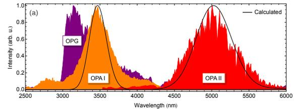
Fig 1. Normalized measured and calculated pulse spectra emerging from successive stages of a compact 2- $\mu\text{m}$  pumped ZGP OPA [1]
