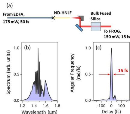
Fig. 1. (a) Scheme for generating a few-cycle 1.55  $\mu\text{m}$  pulse. (b) Spectrum and (c) reconstructed pulse envelope of the few-cycle pulse.
