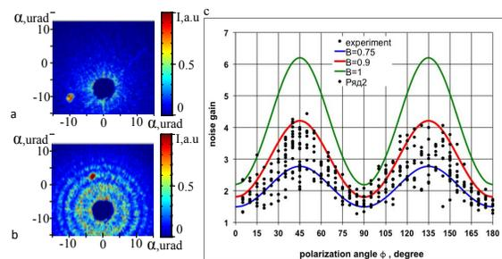
Fig. 1. Angular spectrum of non-amplified (a) and amplified (b) noise; and noise gain vs angle between polarization and crystallographic axis (c).
