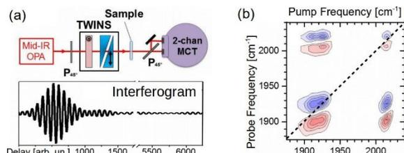
Fig. 1. (a) Scheme of the TWINS-FTIR setup and interferogram of a 6- $\mu\text{m}$  pulse measured at 30% humidity. (b) 2D-IR spectra of the Rhenium carbonyl complex at 0.5 ps delay.
