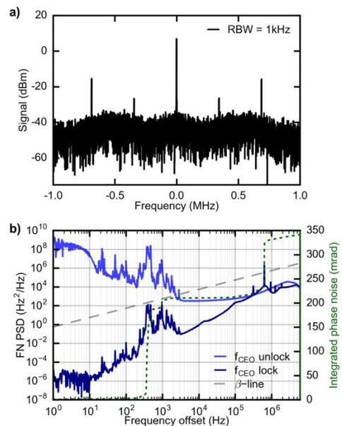
Fig. 1 a) RF spectrum of the CEO beat showing a coherent peak with an SNR of 40 dB at a RBW of 1 kHz. b) Frequency noise power spectral density (FN-PSD) of the CEO beat in free-running (light blue) and stabilized (dark blue) conditions, and corresponding integrated phase noise as a function of the upper cut-off frequency (right axis).
