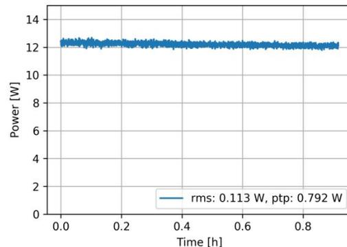
Fig. 1. OPCPA output power as a function of time.
