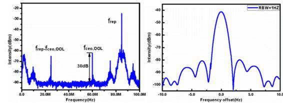
Fig. 2. Spectrum of In-loop and out-of loop f-2f interferometer CEO beat signals.
