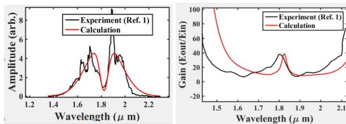
**Figure 1:** (a) The measured input seed to the FOPA1 versus the simulated seed. (b) Spectral gain after amplification in FOPA both experimentally<sup>1</sup> and our simulation.
