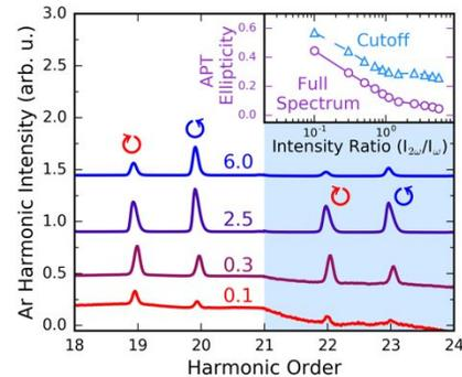
Figure 2. Experimental CPHHG spectra and theoretical ellipticity of the APTs (inset) in Ar for different intensity ratios,  $I_{2\omega}/I_{\omega}$ , of the driving field (experimental ratios given next to spectra).
