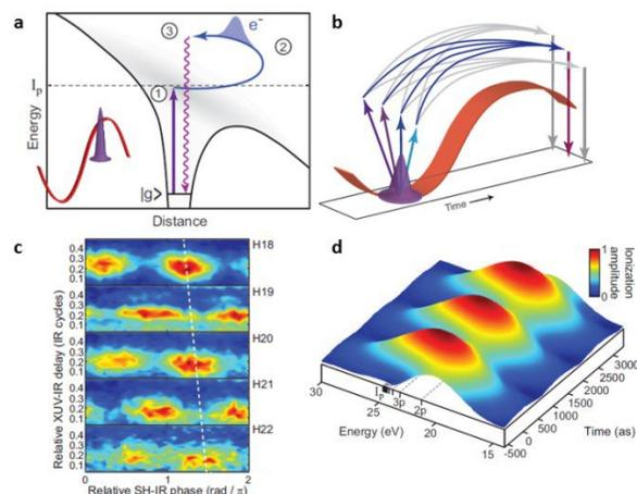
Fig.1. (a) Principle of photoionization self-probing spectroscopy. (b) Interferometer picture of XUV-initiated HHG. (c) Perturbative probing of the HHG dynamics. (d) Reconstruction of the photoionization dynamics in strongly IR-driven helium.
