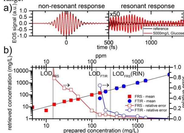
Fig. 1. a) FRS trace of a reference (water, black) and sample measurement (5000 mg/L glucose, red). b) Glucose dilution series: FTIR (blue), FRS (red). The LOD is defined as the concentration at which the relative standard deviation of the retrieved value is 100%.
