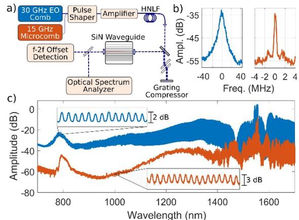
Fig. 1: a) Experimental schematic (HNLF: highly-nonlinear fiber). b) Detected offset frequency of 30 GHz EO comb (left) and 15 GHz microcomb (right) at 775 nm. c) Experimental supercontinuum with comb-mode-resolved regions as insets.
