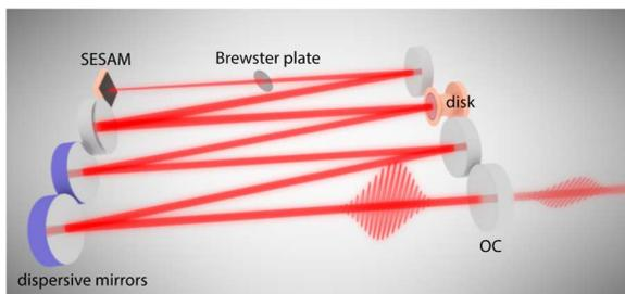
Fig. 1. A high-power modelocked thin-disk laser can deliver hundreds of watts in resonators with similar layout to that of a low power bulk ultrafast oscillator.
