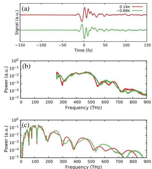
Fig. 1. (a) Temporal waveforms of the single cycle MIR pulses used for the HHG. (b) HHG spectra from silicon thin crystal driven by the single-cycle MIR pulses. (c) Simulated HHG spectra.
