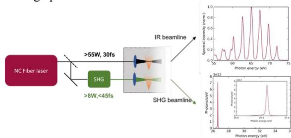
Fig. 1. Simplified experimental together with respective spectra of the generated harmonics (NC – nonlinearly compressed).
