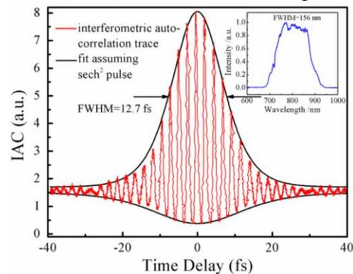
Fig. 2. Interferometric autocorrelation traces. Inset: corresponding the spectrum.
