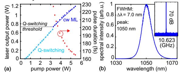
Fig. 2. (a) Laser output power and pulse duration as a function of pump power. (b) Optical spectrum and radio frequency trace (inset) with a span of 5 MHz and a resolution bandwidth of 3 kHz.
