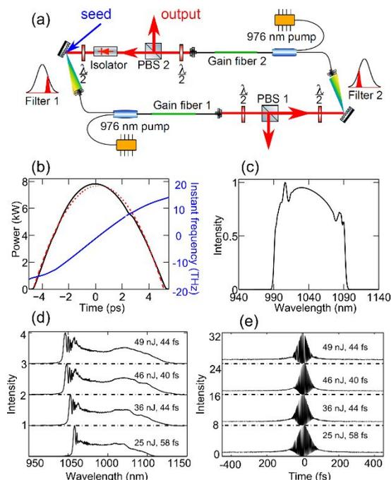
Fig. 1. (a) Schematic of the ring Mamyshev oscillator. The black curve indicates the gain bandwidth and the red curve shows the passband of the filter. PBS: polarizing beam splitter, (b) simulated output temporal profile (black) with fitted parabolic shape (red) and instantaneous frequency (blue) and (c) simulated output spectrum, (d) measured output spectra and (e) autocorrelation traces of the compressed pulses for the indicated energies.
