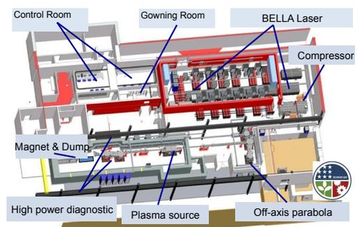
Fig. 1. Layout of the BELLA PW LPA Facility with the Laser, Target and Diagnostics rooms.
