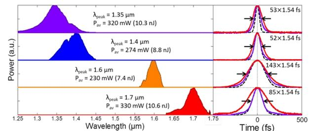
Fig. 3 (Left column) Filtered spectra from 4-cm DCF. Their peak wavelength, pulse energy, and average power are labeled in the figure. (Right column) Autocorrelation traces of the pulses before (red curves) and after (purple curves) being dechirped by fused silica plates. Black dashed curves plot the calculated autocorrelation traces of the transform-limited pulses allowed by the filtered spectra.
