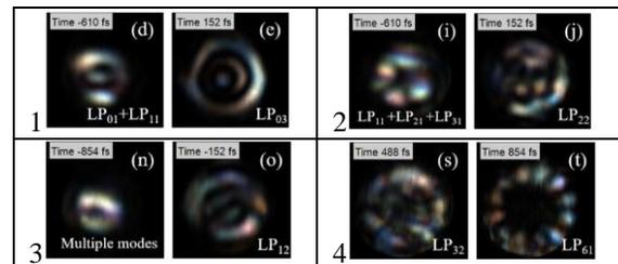
Table 1. Selected snapshots from the STRIPED FISH-measured color movies for four different coupling situations. Snapshots are shown for two times for each coupling situation. Pulses are propagating at the viewer. The color indicates the phase by showing the actual (false) color as would be seen by the eye if it had  $10^{14}$  times faster resolution.
