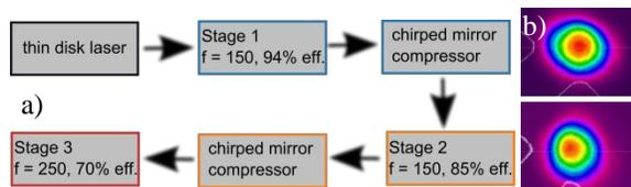
Fig. 1 a) Setup schematics b) Beam Profile at low power, no nonlinear effects (top) and high power throughput (bottom)
