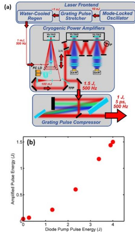
Fig. 1. (a) Layout of the 1 J, 500 Hz, 5 ps laser system. (b) Measured pulse energy exiting the final amplifier at 500 Hz repetition rate as a function of laser diode pump energy.
