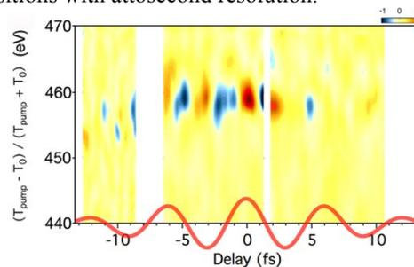
Fig. 1. XAFS spectrum of TiS<sub>2</sub> after excitation with a 1.8-cycle duration field at 1850 nm.
