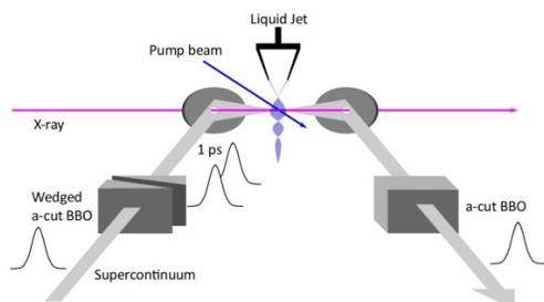
Fig. 1. Schematic experimental setup illustrating the different beam paths for X-rays, interferometric timing tool as well as the optical pump beam to study chemical dynamics in the liquid phase.
