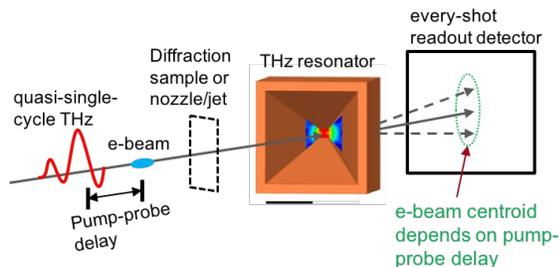
Fig. 1. Schematic of the THz streaking experiment, as well as the concept of a timing tool for pump-probe ultrafast electron diffraction measurement.
