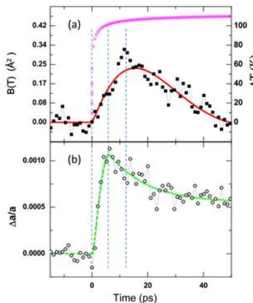
**Fig.1** (a) Transient lattice temperature. The asterisk line is a simulation of Auger relaxation and the solid line is the TTM model fitting. (b) Relative lattice spacing change as a function of time.
