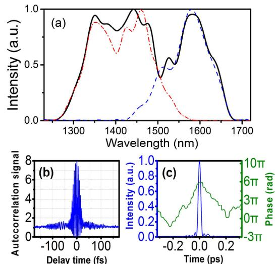
Fig. 2. Spectra, interferometric autocorrelation as well as temporal intensity envelope and phase of the synthesized pulses
