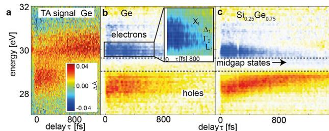
Fig. 1. (a) Typical transient absorption signal at the Ge  $M_{4,5}$ -edge. (b) Retrieved carrier dynamics from (a) featuring hot electron and hole relaxation and recombination (Inset: enlarged conduction band shows valley-specific carrier dynamics). (c) In Si-Ge alloy trapping of electrons in midgap states is observed.
