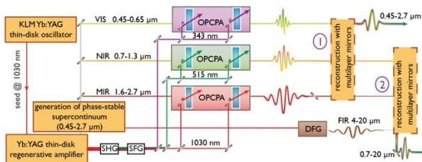
Fig. 1. Schematic architecture of a three-channel OPCPA field synthesizer.
