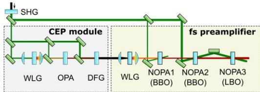
Fig. 1. Schematic of the OPCPA frontend. SHG: second harmonic generator; WLG: white light generator; (N)OPA: (noncollinear) optical parametric amplifier; DFG: difference frequency generator
