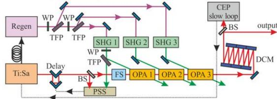
Fig 1. Layout of the system. Ti:Sa: Titanium-sapphire oscillator, Regen: regenerative thin-disk amplifier, BS: beam splitter, WP: waveplate, TFP: thin-film polarizer, SHG: second harmonic generation, PSS: pump-seed synchronization, FS: fused silica stretcher, DCM: double-chirped mirror compressor.
