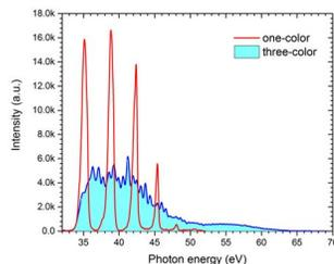
Fig. 1. Harmonic spectrums from Ar gas cell
