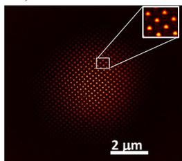
Fig. 1. XUV beam profile at the focus characterized by coherent diffractive imaging of a uniform array of holes.
