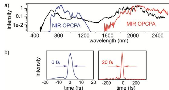
Fig. 1. a) CEP stable supercontinuum (black) amplified portion of the spectrum in the NIR channel (blue) and in the MIR channel (red). b) Compressed pulses of the NIR (blue) and the MIR channel (black).
