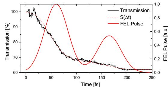
Fig. 1. An example of a time-resolved optical transmission signal from a seeded FEL with a detuned  $R_{56}$  (solid black line) and the resulting fit ( $S(\Delta t)$ , dashed red line). From the fit, the temporal structure of the FEL pulse is reconstructed (solid red line). For more experimental details see [4].
