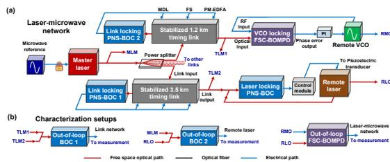
Fig. 1 (a) Laser-microwave network (VCO, voltage-controlled oscillator); (b) Out-of-loop characterization setups<sup>4</sup>.
