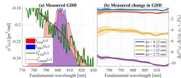
Fig. 2. (a) Measured fundamental and SHG spectra and retrieved GDD. (b) Measured change in GDD as stretcher grating separation is tuned (shaded regions indicate estimated standard error).
