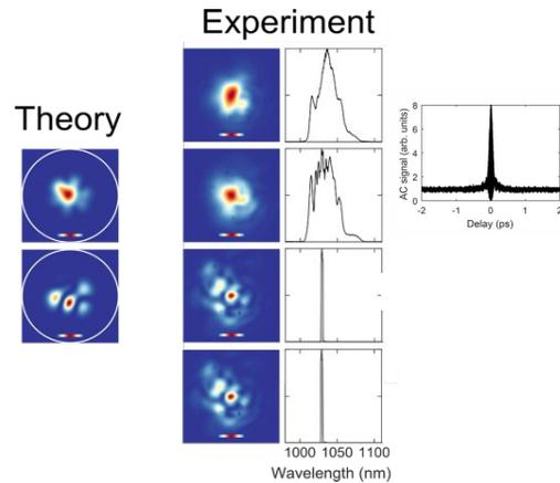
Fig. 1. Theoretical and experimental spatial and spectral profiles, and autocorrelation of modelocked state.
