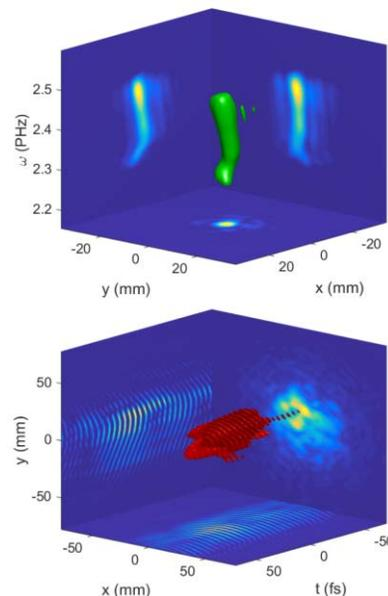
Fig. 1. Reconstructed spatio-spectral amplitude profile (top), reconstructed spatio-temporal electric field, slightly after focus (bottom).
