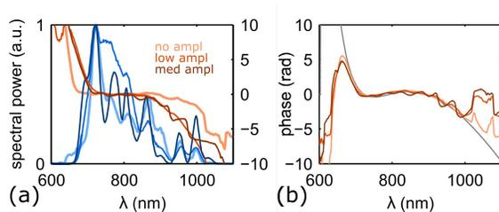
Fig. 1. Spectral phase measurement of (a) seed and amplified pulses, and (b) comparison of the parametric phase with theoretical value for phase-mismatch. Darker colors correspond to larger gain.
