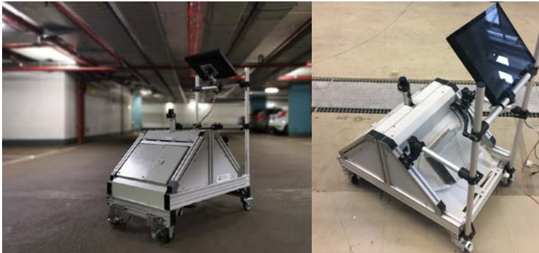
Figure 1: The mobile platform with its operating panel. The laser scanner, used to localize the system is at the top of the device. The camera, used for crack detection is not visible because it is under the system, acquiring the parking ground.
