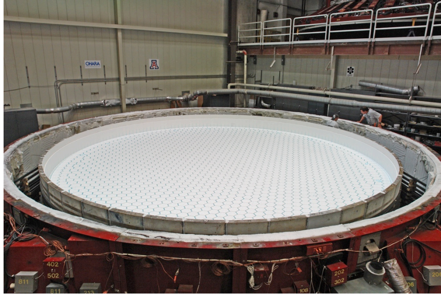
Figure 10. Mold for GMT Segment 2 (same for all off-axis segments) surrounded by the lower part of the furnace. The furnace lid can be seen at top right on its storage shelf. Photo by Ray Bertram, Steward Observatory.
