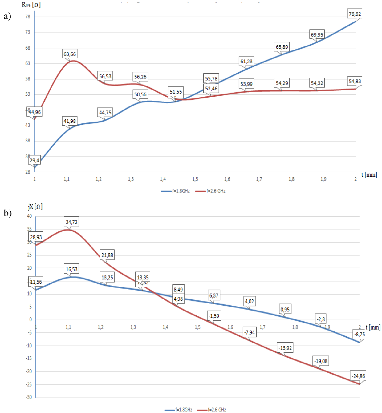
Figure 4. List of characteristics of dielectric thickness influence on input impedance for f_0 = 1.8 GHz and f_0 = 2.6 GHz: a) real part b) imaginary part.
