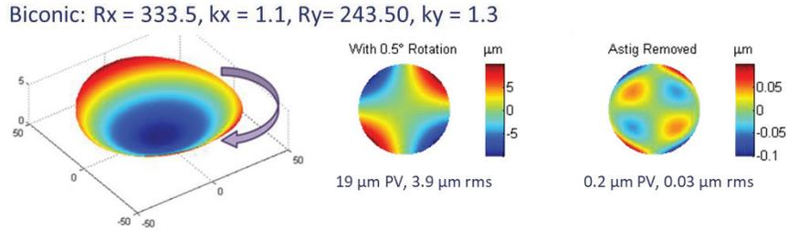
**Figure 4: Simulation on a biconic 100 mm circular aperture. A rotational offset of  $0.5^\circ$  causes 19  $\mu\text{m}$  of PV astigmatism.**
