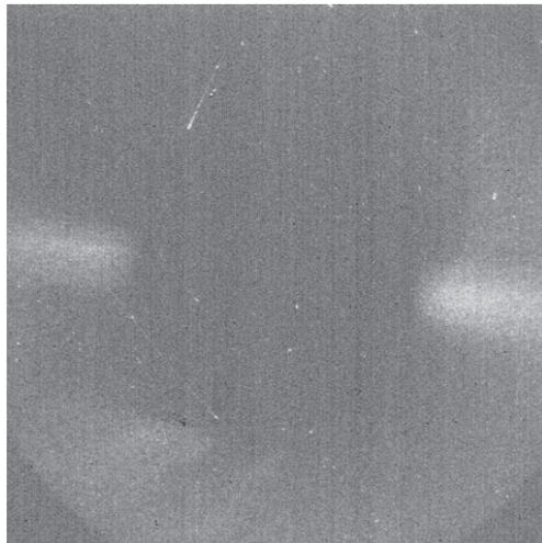
Figure 9. UV first light confirms a misalignment of the occultation system. Stray light pattern is visible in the third quadrant of the image.
