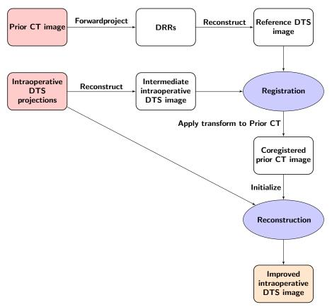
Figure 2. Flowchart of the proposed reconstruction method.
