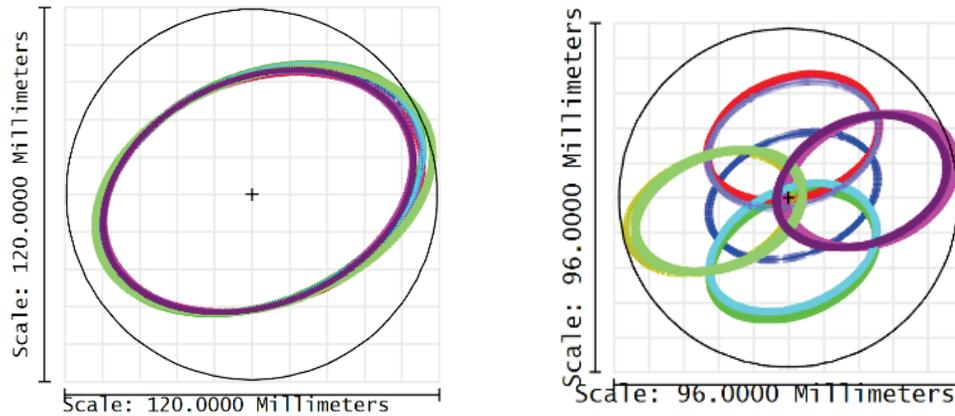
Figure 9. Footprint of different fields on M1 (left) and on M5 (right).
