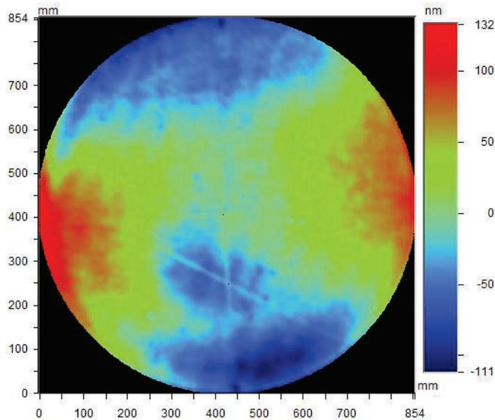
Figure 19. Derotator FM1 WFE measurement (central field of view). WFE RMS: 46 nm.
