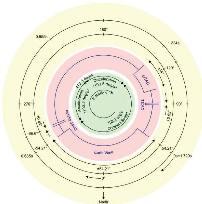
Figure 2. METImage observation principle.
