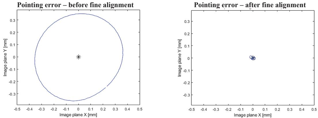
Figure 15. Derotator fine alignment example (FM1).
