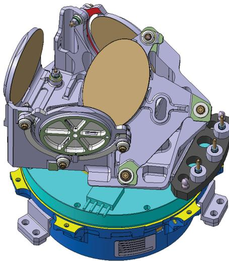
Figure 3. METimage Derotator Assembly (including mechanism, courtesy of Airbus Defence & Space).
