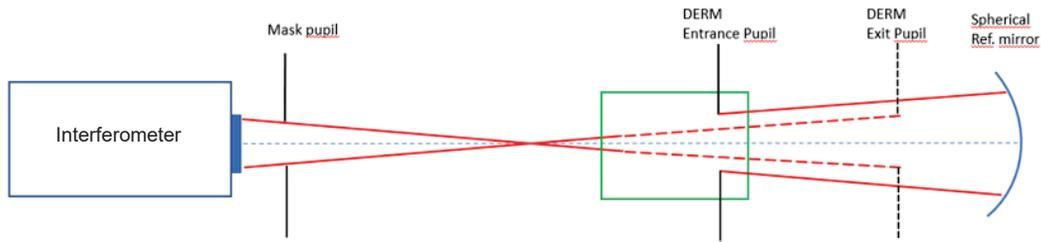
Figure 18. Derotator WFE test setup.
