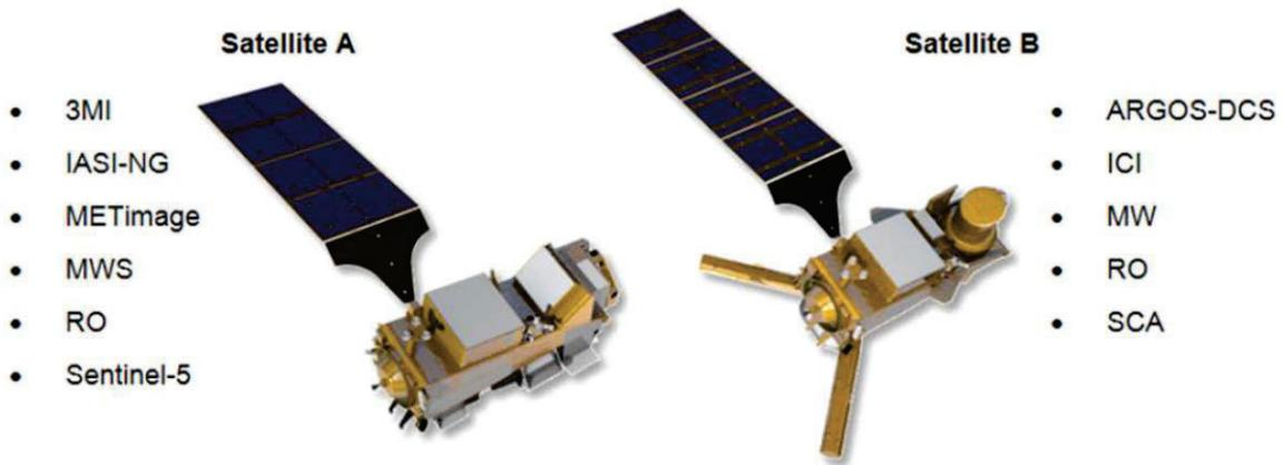
Figure 1. MetOp-SG, the two-satellite space segment of EUMETSAT’s EPS-SG mission.
