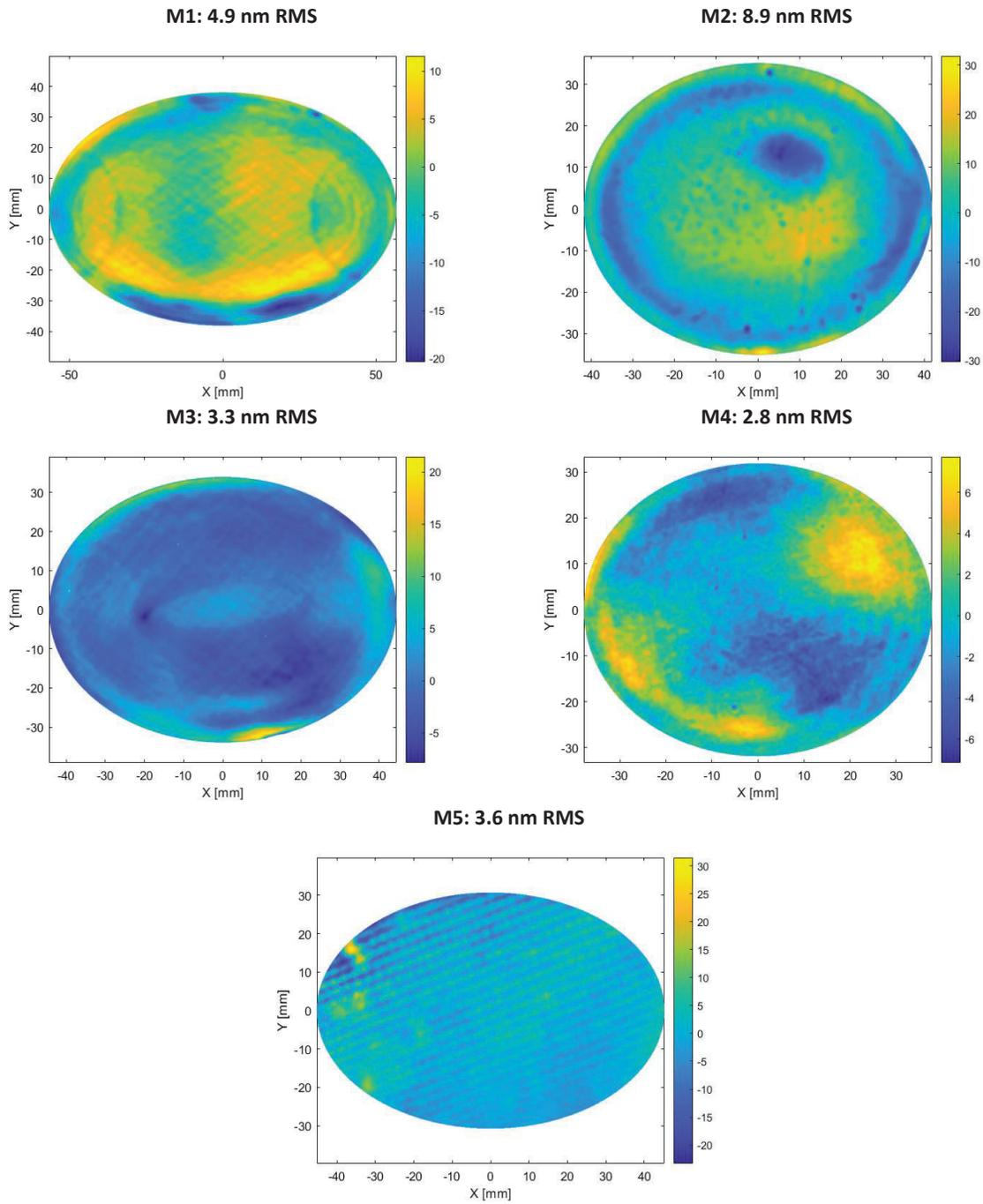
Figure 13: FM1 mirrors measured surface figure error (colour scale units: nm).
