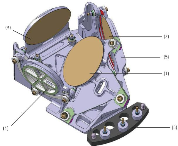
Figure 4. Derotator Optical Assembly.
