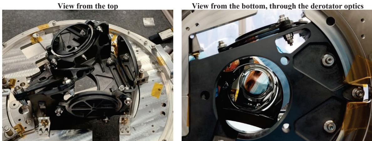
Figure 16. Derotator FM1 re-assembly with coated mirror.
