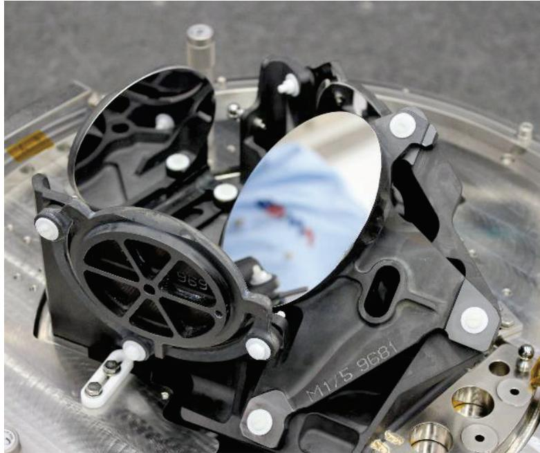
Figure 14: Derotator FM1 assembled and ready to be aligned/tested with the OGSE.
