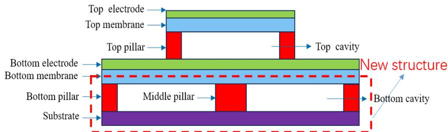
Figure. 2 Double-layer CMUTs structure
