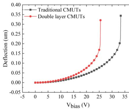
Figure. 4 Center deformation under different bias pressures
