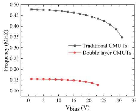
Figure. 5 Resonant frequencies for different bias voltages
