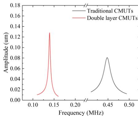
Figure. 6 Amplitude at resonant frequency
