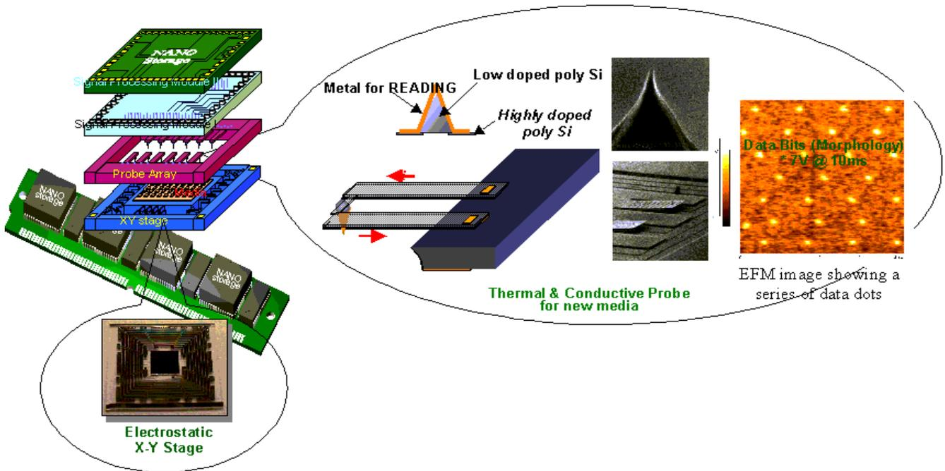
Figure 5. Next generation mobile/micro storage system.
