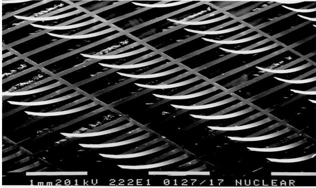
Figure 7a. Bulk micromachined microfin array.
