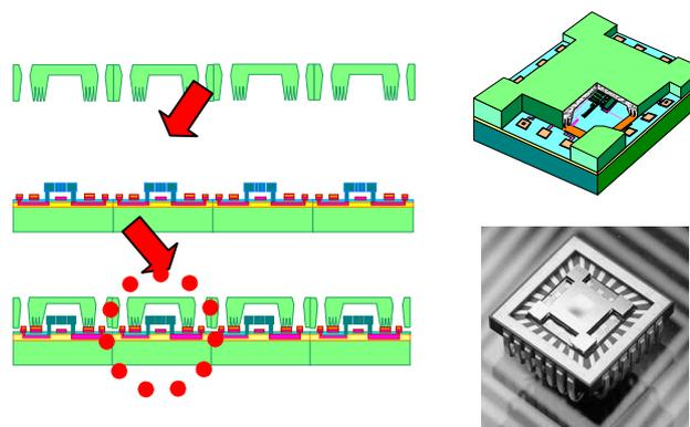
Figure 2b. Wafer-level vacuum packaged micro gyroscope
