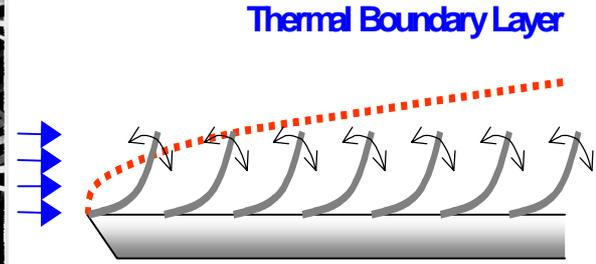
Figure 7b. Breaking up of the thermal boundary layer.
