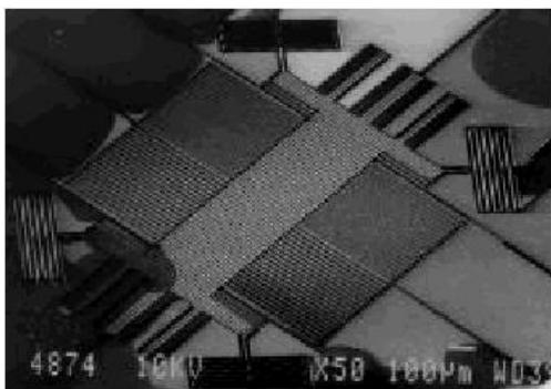
Figure 2a. Silicon-on-Glass processed gyroscope.
