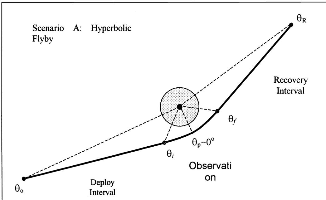
Figure 2. Hyperbolic Flyby. Probes are released from mothership at true anomaly  $\theta_o$ . Probes are required to be at specified relative state when mothership reaches true anomaly  $\theta_i$ . Probes free-fall while sensors point to and observe target region. Observation ends when mothership reaches true anomaly  $\theta_f$ . Probes compute optimal trajectory and return to mothership for recovery.
