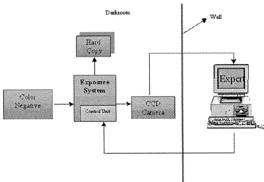
Figure 7: Automated process of enhancing an analog image.
