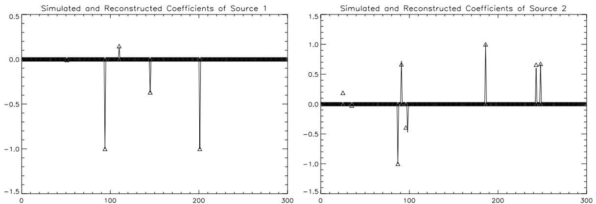
**Figure 8.** On the left, the simulated ( $\Delta$ ) and reconstructed (using ICA-MCA) coefficients of source 1. On the right, the simulated ( $\Delta$ ) and reconstructed (using ICA-MCA) coefficients of source 2. Each decomposition is achieved on the whole dictionary : samples 0 to 149 correspond to the Dirac basis and samples 150 to 299 correspond to the DCT basis. Due to the scale indeterminacy discussed previously, only their relative amplitudes of the coefficients are significant.
