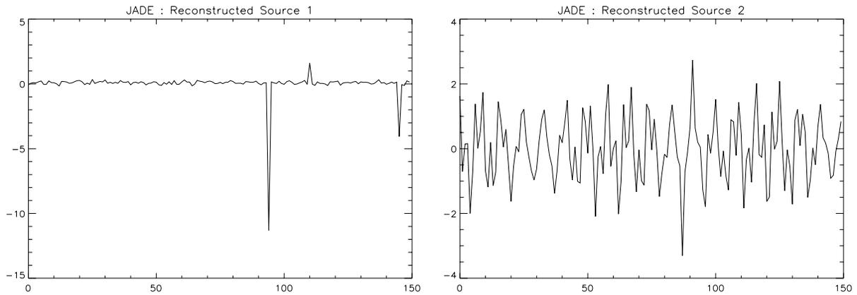
**Figure 7.** The top figures are the two observed data. Each channel is a linear combination of the two sources plus some Gaussian noise. At the bottom, the sources estimated using JADE. One can notice that the low frequency sinusoid of the first source is not well detected. In the middle, the figures show the sources estimated using ICA-MCA; the base line of the second source is now well estimated.
