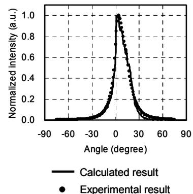
Fig. 7 Luminance distribution of the HSOT II against the viewing angle.
