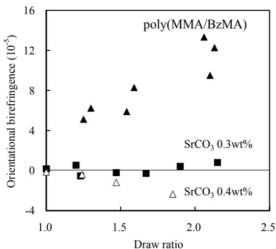
Fig. 9 Orientational birefringence of the poly(MMA/BzMA) films containing SrCO<sub>3</sub> with respect to draw ratio.
