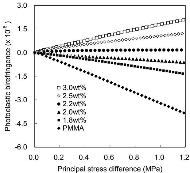
Fig. 11 Photoelastic birefringence of PMMA samples doped with *trans*-stilbene against the principal stress difference at a wavelength of 633 nm.
