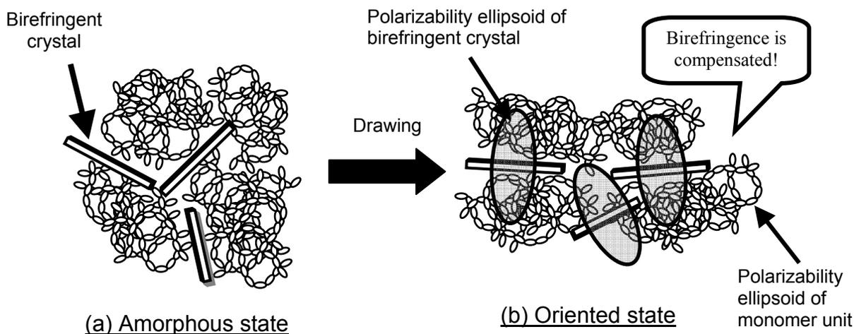
Fig. 8 Mechanism for the compensation of orientational birefringence by the birefringent crystal dopant method. (a) In the completely amorphous state, polymer chains and birefringent crystals are randomly oriented, so that the polymer containing the birefringent crystals exhibits no birefringence. (b) Polymer chains and birefringent crystals are oriented in the drawing direction. However, birefringence of the polymer is compensated by that of the crystal.
