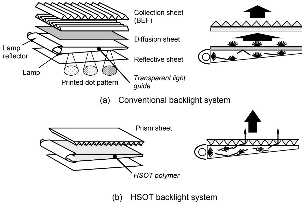
Fig. 5 Schematic diagrams of the HSOT backlighting system and a conventional backlighting system.
