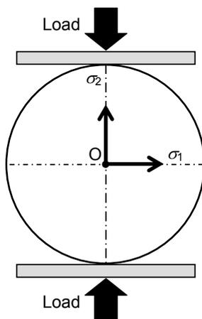
Fig. 10 Experimental set-up of the photoelastic birefringence measurement. Photoelastic birefringence is measured at the center of cylinder-shaped samples under a compression load.
