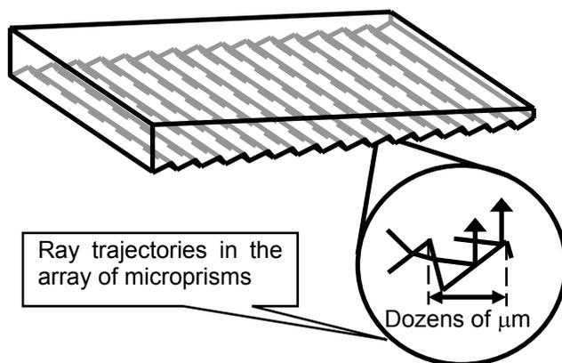
Fig. 6 A schematic diagram of the HSOT II backlight and its luminance distribution.
