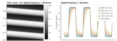
Effect of calibrated CDM model on periodic patterns. Contrast at different spatial frequencies is computed from cross sections shown on the right.
