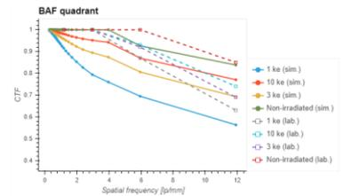
Comparison of measured (dashed line) and simulated (solid line) CTF for different signal level of input patterns
