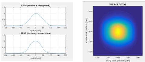
Optical point spread function, including CTE effect after exposition to a proton dose of 9.7 × 10<sup>9</sup> p<sup>+</sup>/cm<sup>2</sup>
