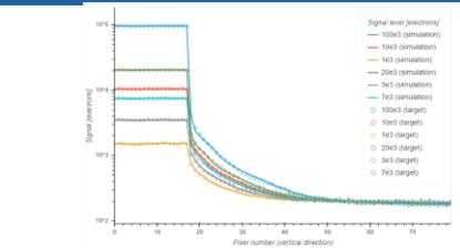
The target test data from laboratory measurements (circles) and the simulated charge profiles (lines) after calibration, showing the distinct charge trails and giving a visual impression of how well CDM can fit the FLEX test data over a wide range of signal level.
