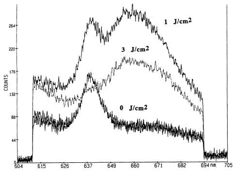
Fig. 11 Cell irradiation resulted in the formation of a new fluorescence band at 600 - 670 nm due to photoproduct formation
