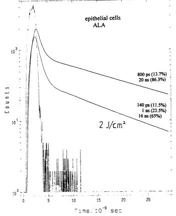
Fig. 12 Photoinduced shortening of the fluorescence decay kinetics. The short component of 800 ps in ALA-incubated epithelial cells can be explained by short-lived naturally-occurring fluorophores
