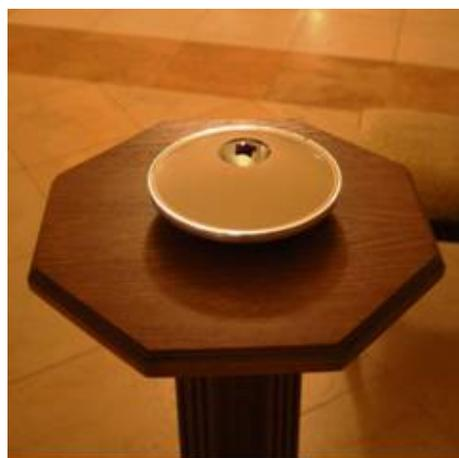
Fig.2. 3D illusion formed by two parabolic mirrors
