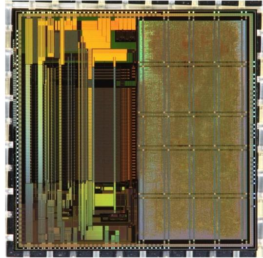
Figure 9: Photograph of the ASIC, view on the top metal layer.
