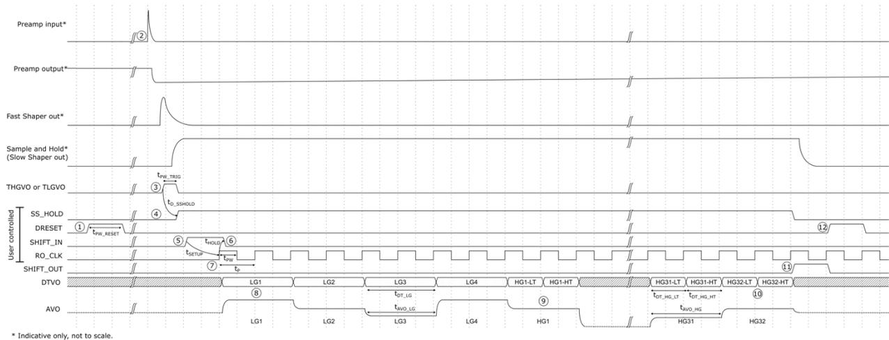
Figure 5: Timing diagram of the track-and-hold readout from slow shapers.
