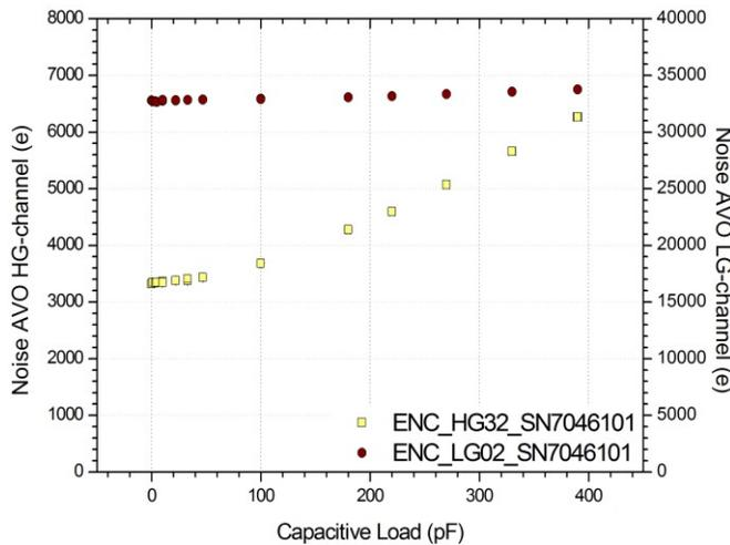
Figure 14: Measurement of the equivalent noise charge versus capacitive load at the pre-amplifier inputs in low-gain (red circles, right y-axis) and high-gain channels (yellow squares, left y-axis).
