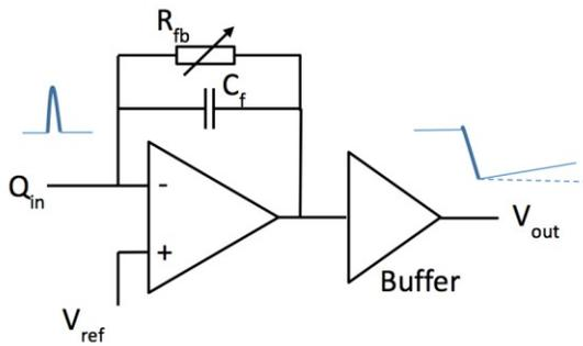
Figure 3: Pre-amplifier principle.
