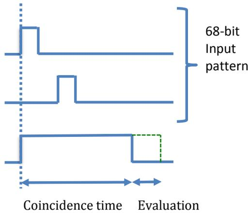
Figure 6: Illustration of two digital pulses within the coincidence time duration.
