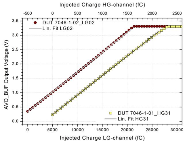
Figure 13: Measurement of the output voltage at AVO\_BUF versus injected charge for a high-gain (yellow squares) and a low-gain channel (red circles) with linear fits (lines).
