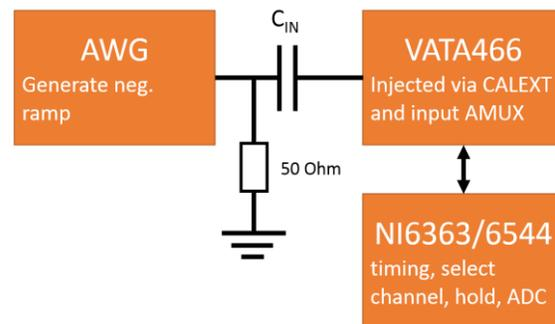
Figure 11: Block diagram of the system used for charge injection in all test cases but for coincidence measurements.
