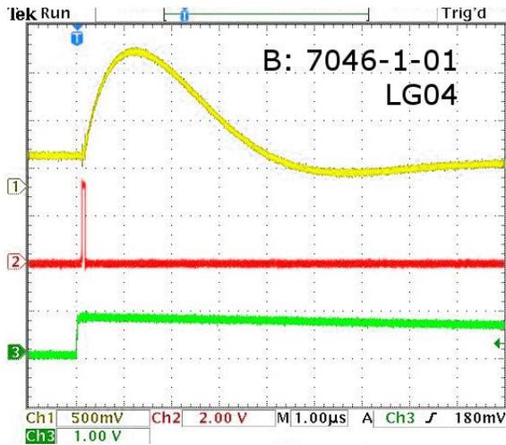
Figure 12: Oscilloscope screenshot with DUT1. The charge of 8 pC was injected into low-gain channel LG04. The yellow line (1, top) shows the slow shaper output, the red line (2, middle) the trigger output and the green line (3, bottom) the input signal.
