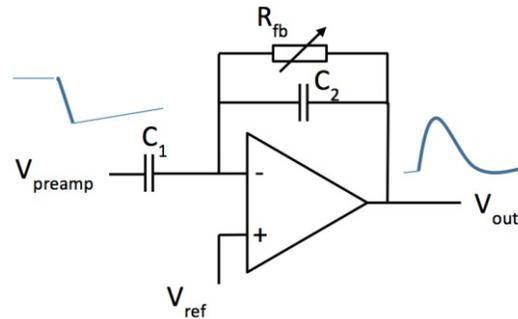
Figure 4: CR-RC shaper principle.
