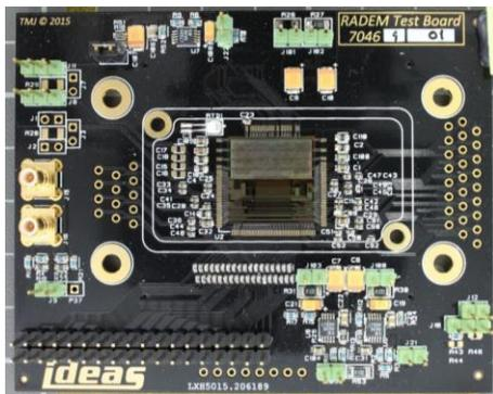
Figure 10: Photograph of the ASIC on a test card, top view.
