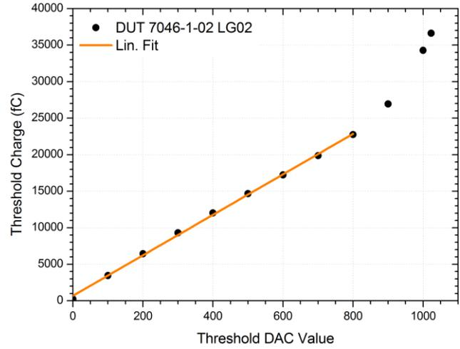
Figure 16: Calibration of the threshold charge over threshold DAC value in a low-gain channel.
