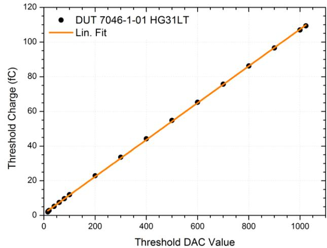
Figure 18: Calibration of the threshold charge over threshold DAC value for a high-gain low-threshold (HGLT) channel.
