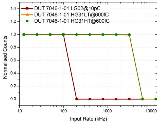
Figure 19: Measurement of the normalised counts versus input rate in a low-gain channel (red), and a high-gain channel (HGLT orange and HGHT green).
