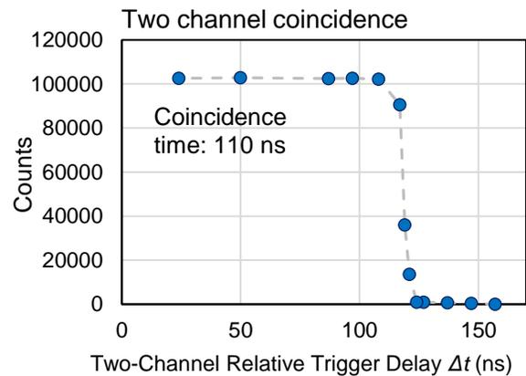
Figure 21: Measurement of the counts versus relative trigger delay between the two channels.
