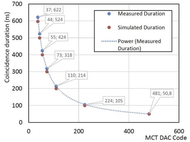
Figure 7: Measurement and simulation of the programmable code and the coincidence time duration.
