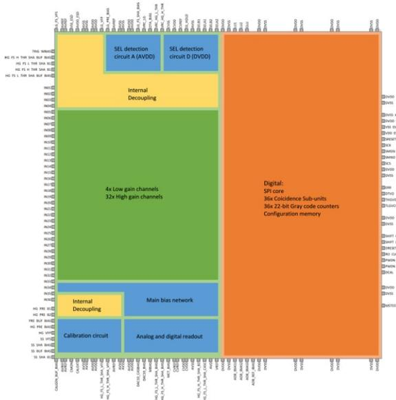
Figure 8: Floor plan with signals and pad frame.
