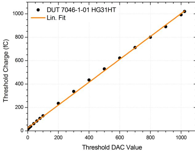
Figure 17: Calibration of the threshold charge over threshold DAC value in a high-gain high-threshold (HGHT) channel.
