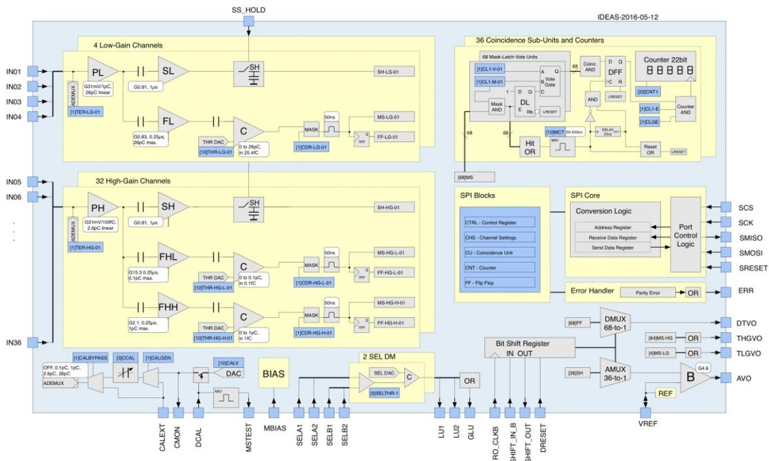
Figure 2: ASIC block diagram.
