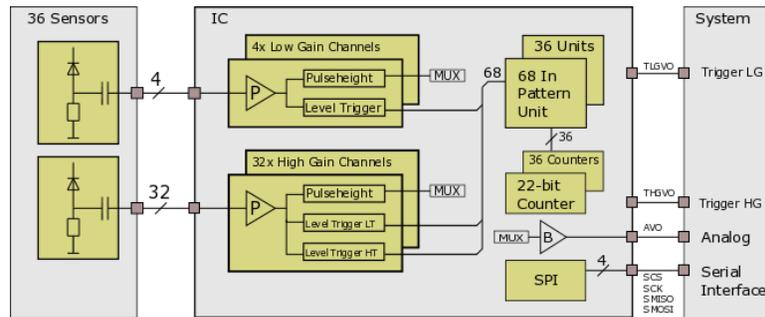
Figure 1: Block diagram with radiation sensors (left), the integrated circuit (ASIC, centre), and readout system (right).
