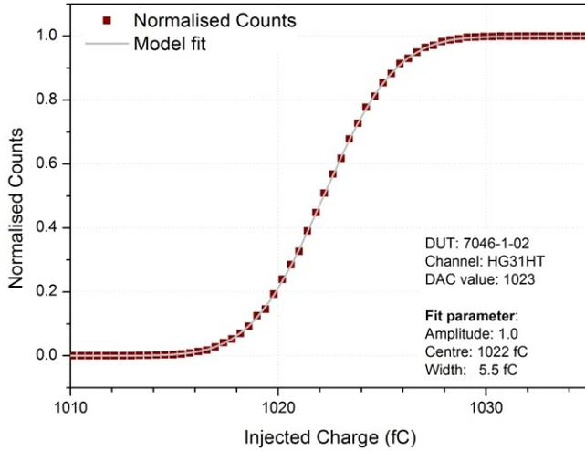
Figure 15: Measurement of normalised counts versus injected charge. The data is fit by an error function.
