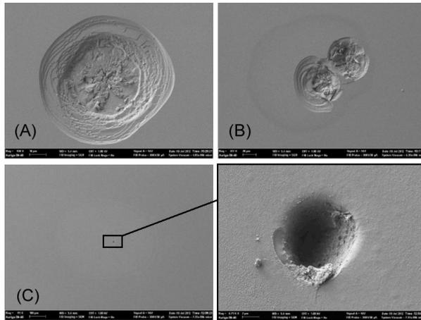
Figure 3. Typical damage morphology induced by laser irradiation with a fluence of (A)  $39.2 \text{ J/cm}^2$  (p-polarized light), (B)  $53.5 \text{ J/cm}^2$  (p-polarized light), and (C)  $61.4 \text{ J/cm}^2$  (s-polarized light).
