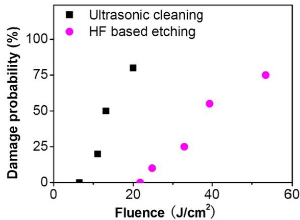
Figure 4. Damage probability of polarizer coating deposited on substrate cleaned by different cleaning methods.
