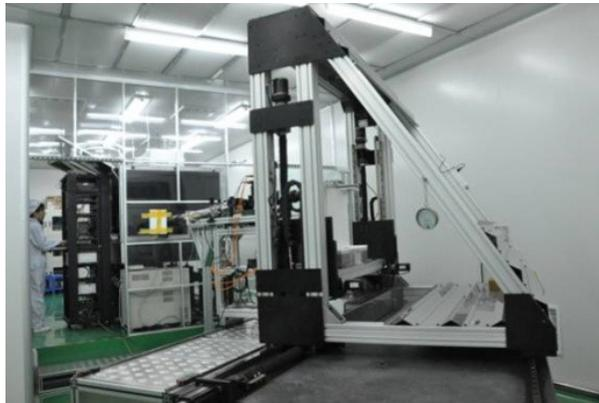
Figure 6. The picture of the platform for off-line laser conditioning
