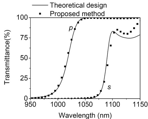
Figure 2. Theoretical and experimental spectra of a design monitored by proposed method.
