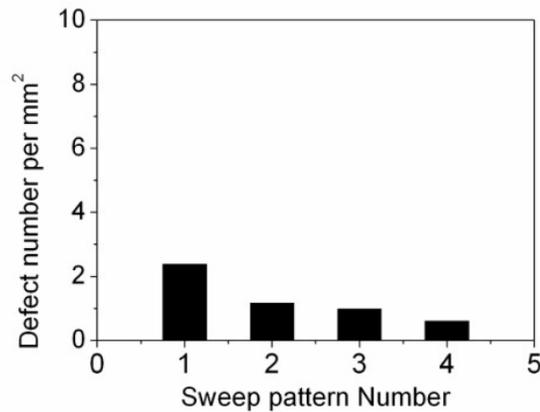
Figure 5. Influence of sweep pattern on defect density of multilayer coatings.
