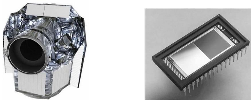
**Fig. 1.** (Left) CHEOPS. (Right) Back-illuminated CCD sensor
