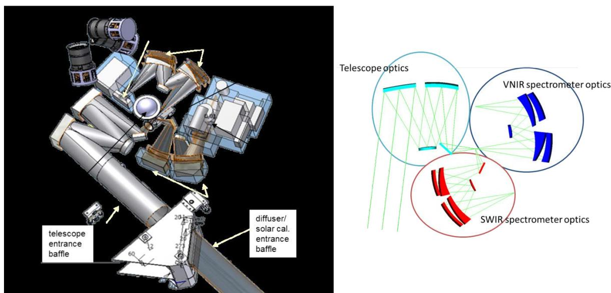
**Fig. 3.** Left: Basic concept of the instrument optics. Right: optical layout of telescope and spectrometers (not showing calibration).
