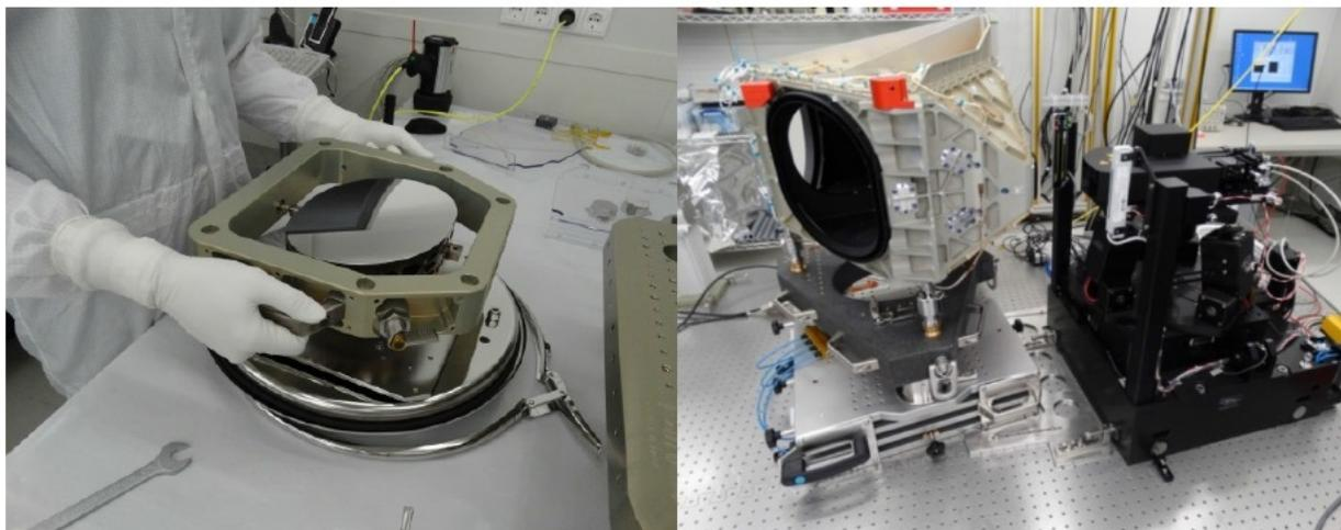
**Fig. 4.** Optical flight components of the telescope. Left: An individual mirror of the TMA. Right: The telescope during its alignment (together with its dedicated optical ground support equipment).
