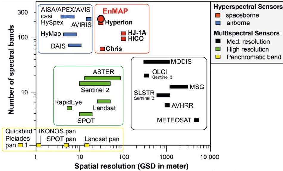
Fig. 1. Overview of the spectral and spatial resolution of selected airborne and spaceborne hyperspectral and multispectral sensors [1].
