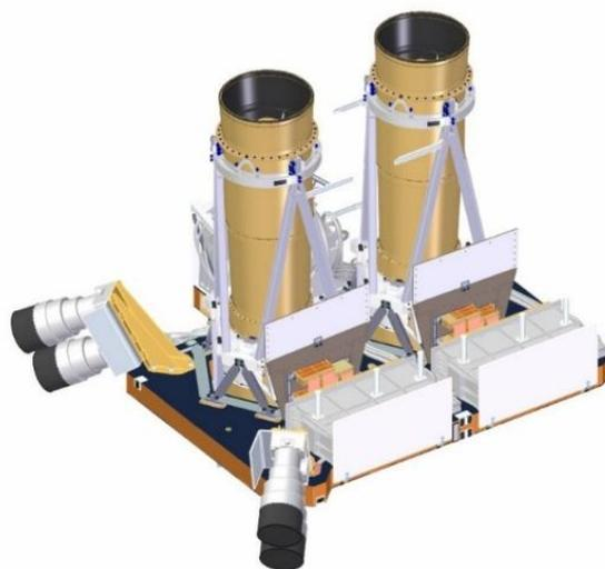
**Fig. 1.** 3D view of the Ingenio/SEOSAT primary payload
