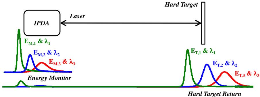
**Fig. 1.** 2- $\mu$ m triple-pulse IPDA lidar principle of operation for simultaneous atmospheric CO<sub>2</sub> and H<sub>2</sub>O measurement. The energy of each transmitted pulse is monitored inside laser enclosure. The wavelength of each pulse can be tuned and locked independently to any position around the CO<sub>2</sub> R30 line. One wavelength criteria for minimizing molecular interference errors is presented in Fig.2.
